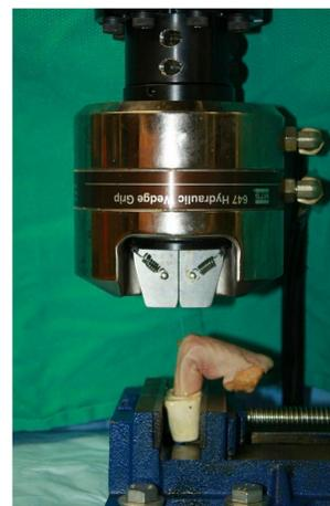
Figure 3: Experimental testing fixture showing specimen in bone cement fixed to the base of the testing machine. Suture attached to vertical actuator grips for tensile loading at a rate of 100mm/min.
