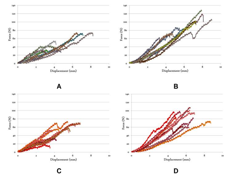
Figure 4: Force-displacement plots of middle and index fingers prepared with JuggerKnot anchor plus suture (anchor) and suture only (suture) through transverse bone tunnels. A. anchor middle, B. suture middle, C. anchor index, and D. suture index.
