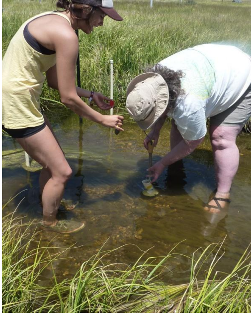
Figure 4: The sampling procedure in the EFJR involved sinking a coring apparatus 2 cm into the sediments and aspirating the contents into sterile tubes .
