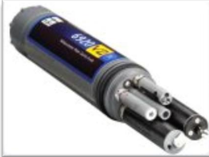
Figure 5: The continuous monitoring equipment set up in the EFJR (left) includes a SONDE (YSI, Inc., Ohio, USA ), a SUNA UV nitrate sensor (SATlantic LP, Halifax, Canada) and a Cycle-P phosphate sensor (Wet Labs, Oregon, USA). At the right is a photo of a SONDE that collects temperature, pH, dissolved oxygen, specific conductivity, and turbidity data at 15-minute intervals.
