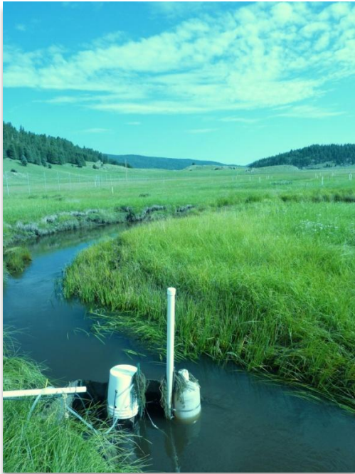
Figure 5: The continuous monitoring equipment set up in the EFJR (left) includes a SONDE (YSI, Inc., Ohio, USA ), a SUNA UV nitrate sensor (SATlantic LP, Halifax, Canada) and a Cycle-P phosphate sensor (Wet Labs, Oregon, USA). At the right is a photo of a SONDE that collects temperature, pH, dissolved oxygen, specific conductivity, and turbidity data at 15-minute intervals.
