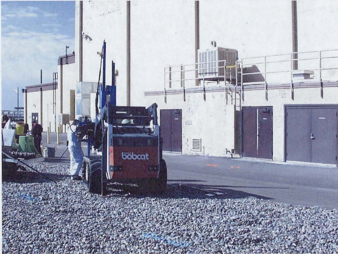
Figure 3.3-1 Collecting soil samples with the Geoprobe™ from beneath the Building 6597 drywell, located in the gravel area near the edge of the asphalt pavement. View to the southwest. September 26, 2002
