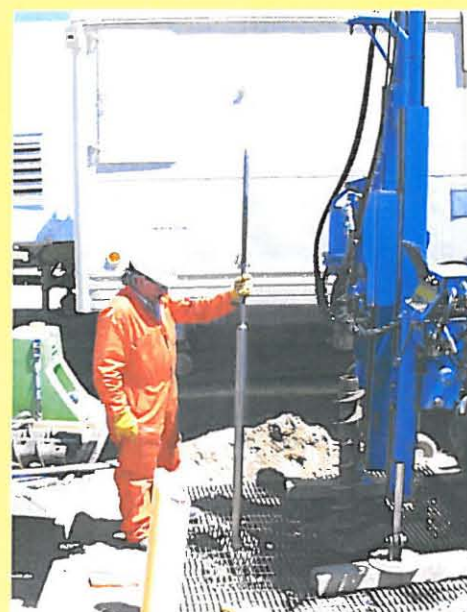
Three-foot long Geoprobe soil sampling device used to collect soil samples.
