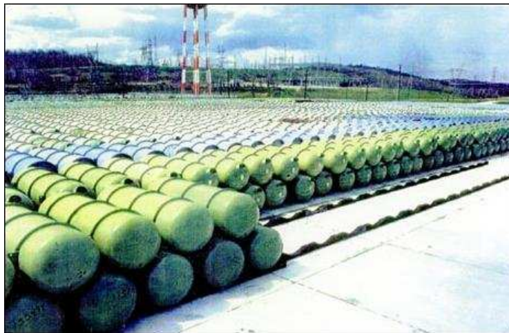
DUF 6 Cylinder Storage Yard at the Portsmouth, Ohio Gaseous Diffusion Plant [ANL 2013]
