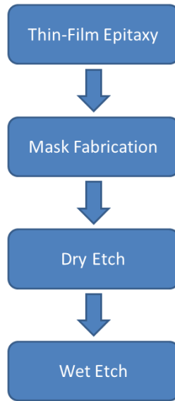
Figure 3.1 The main steps of the top-down etch technique for fabricating GaN nanostructures.
