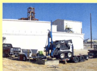
Collecting soil samples with the Geoprobe.
