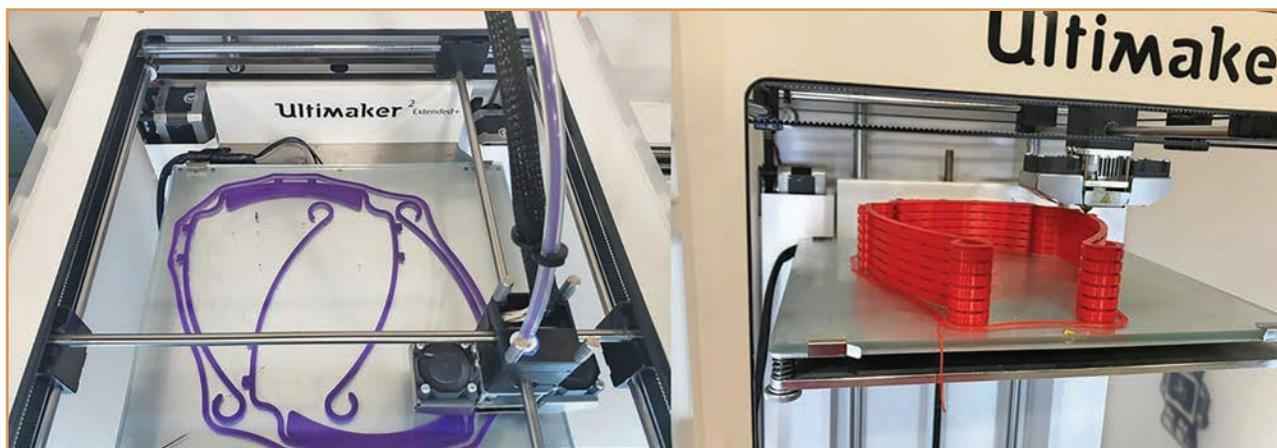
**Figure 2.** The 3DVerkstan 3D printed face shield headband design printed with polylactic acid filament. This design is universal in size and was primarily distributed to first responders and healthcare providers. (Left) A single layer of two headbands printed simultaneously. (Right) A modified stereolithography (.stl) to print stacked headbands for increased productivity and print efficiency.
