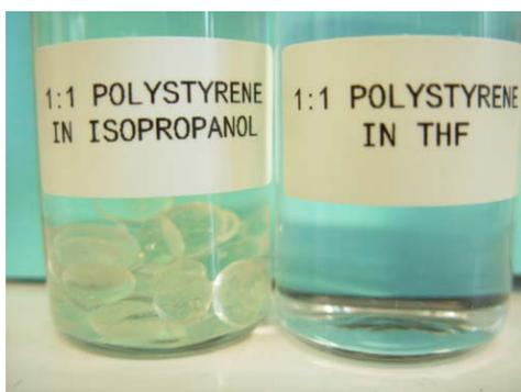
**Figure 11 Solubility test of polystyrene (polymer) in isopropanol and THF (solvent)**
