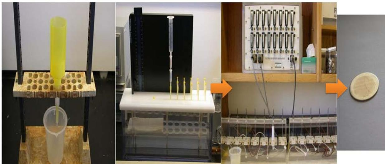
**Figure 3 Ion exchange process, extraction chromatography, electrodeposition, and electrodeposited steel plate**
