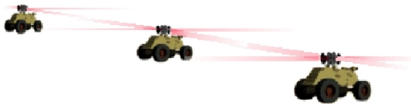
Figure 1: The role envisioned for the UGVs. Their four motion detection sensors can pivot around a vertical axis, so that the sensors can point independently of the vehicle’s orientation. When appropriately configured, they can create a “virtual fence,” capable of detection of motion to and from an area of interest.
