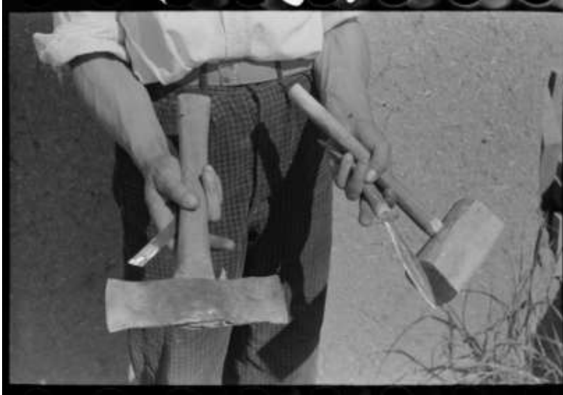
Title: Handmade tools of Spanish-American farmer at Chamisal, New Mexico. The axe was made by welding two automobile spring leaves together and then sharpening; the dagger was filed down from a piece of automobile spring leaf and inserted in the bone handle. Creator(s): Lee, Russell, 1903-1986 , photographer
