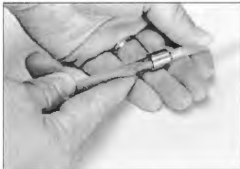
Figure 1. Attaching tubing to the sampling implant.
