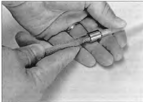
Attaching polyethylene tubing to the sampling implant.
