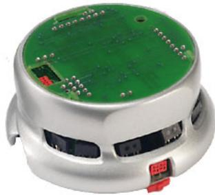
Figure 5.2: The Khepera II mobile Robot
