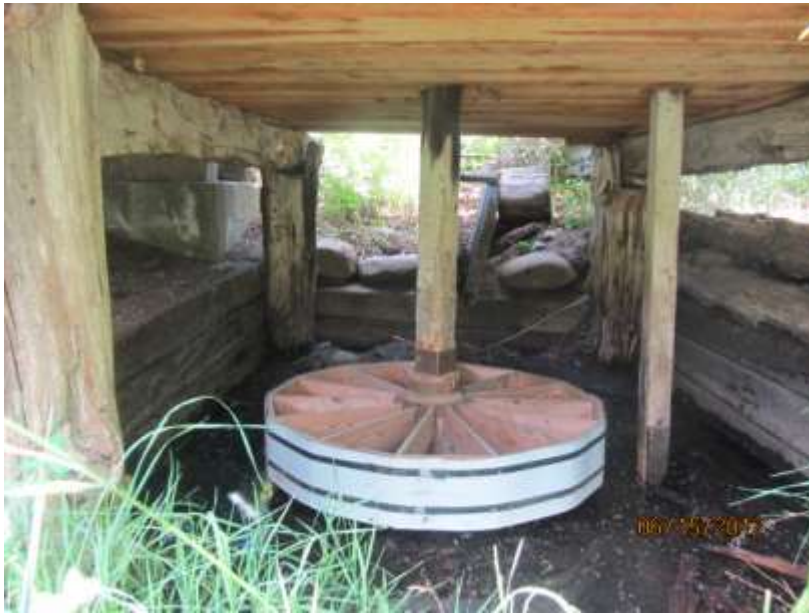
Traditional molino at Córdoba family property in Vadito NM. Renovated horizontal wheel after remodel June 2012
