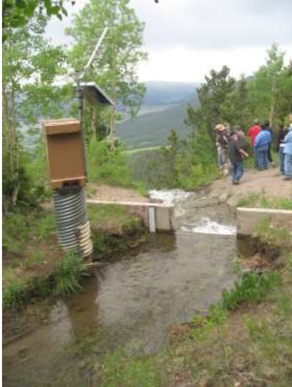
Trans-Basin Acequia de la Presa Waterfall Gauge and Headgate for Chacón. June 2007
