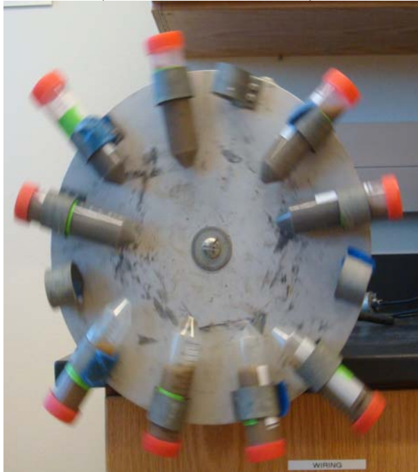
Figure 29. Samples placed in mixer for leach tests
