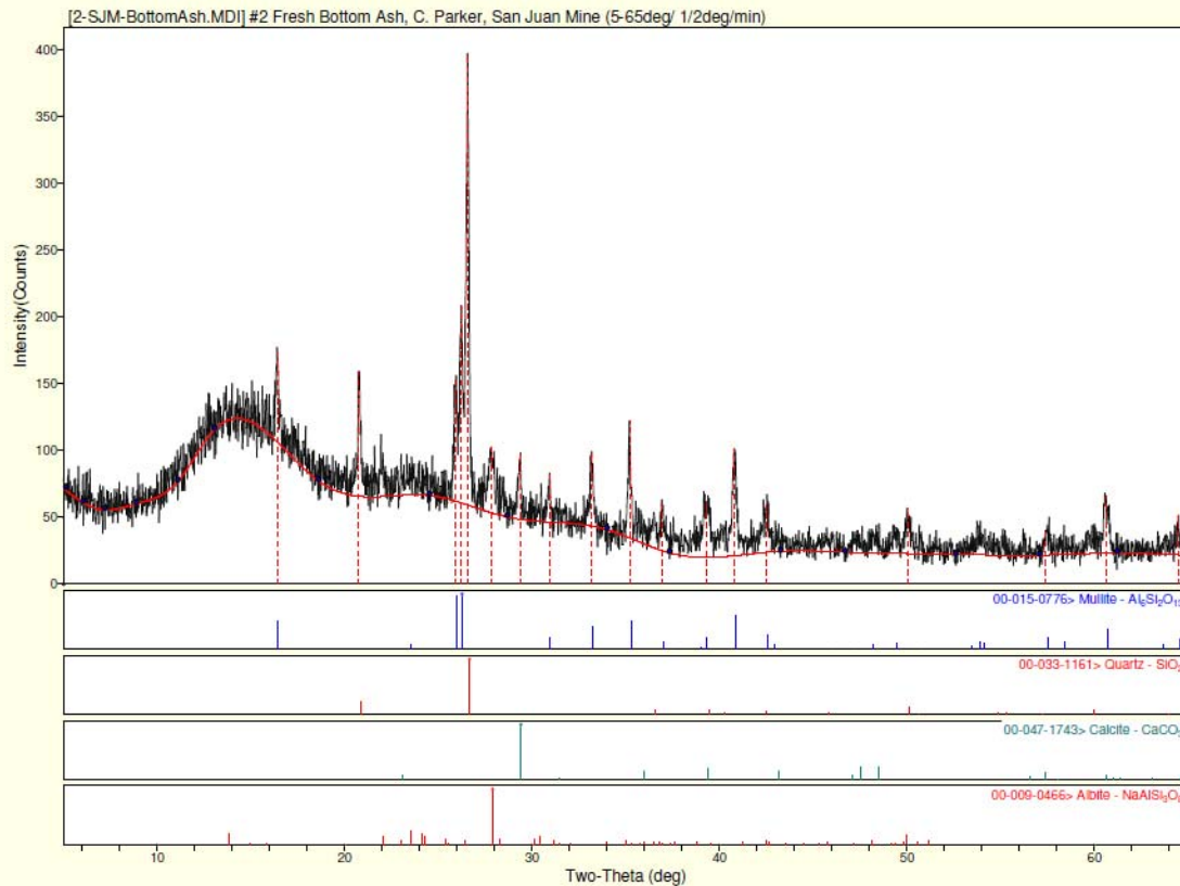
Figure 62. XRD pattern for fresh bottom ash. The library patterns are for mullite (top), quartz (second from top), calcite (third from top) and albite (bottom).
