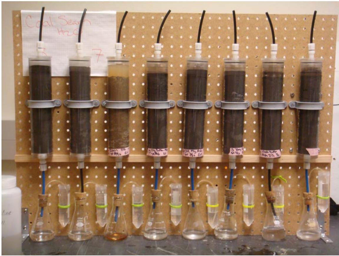
Figure 30. Photo of 2 in ID by 10 in tall columns used in column leach studies.
