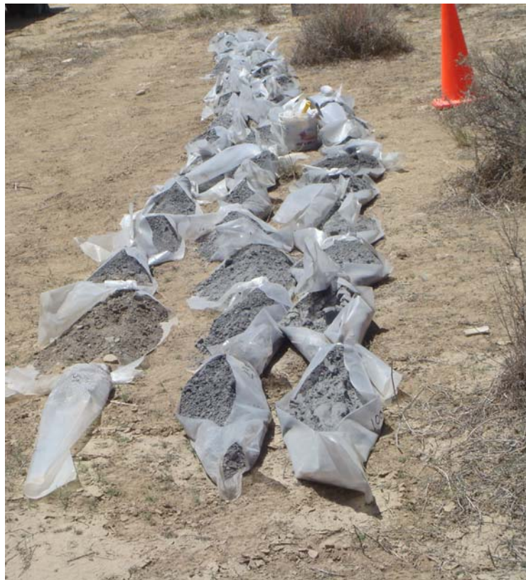
Figure 26. Example photo of core samples from sonic drilling.
