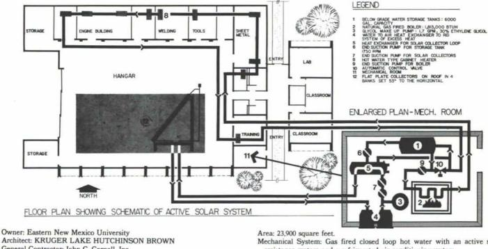
General Contractor: John C. Cornell, Inc. Construction: Load bearing masonry and steel bar joist. Mechanical System: Gas fired closed loop hot water with an active solar assistance system and a refrigerated air conditioning system. Cost: \$1,028,644.00.
