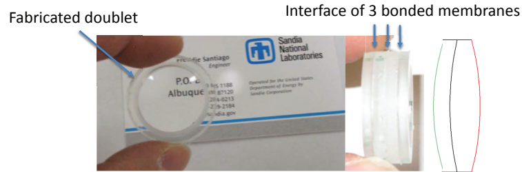
Figure 1.11: Fabricated APLD under constant volume condition.
