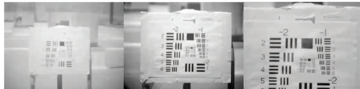
Figure 4.9: Images at the three different states of an Air Force resolution target at 15 meters.
