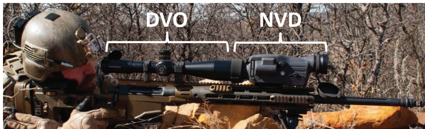
Figure 4.14: Operator demonstrating "in-line" configuration of DVO and NVD (Image courtesy of DRS Technologies)
