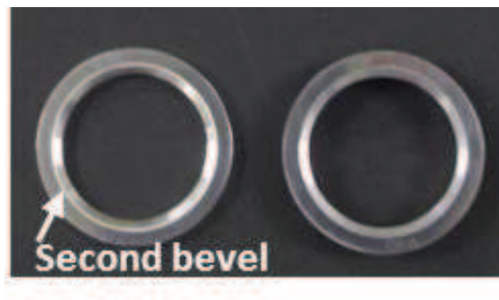
Figure 2.33: Finished polished thin (Left) and thick (Right) Al rings showing the second bevel as lighter color indicated by arrow
