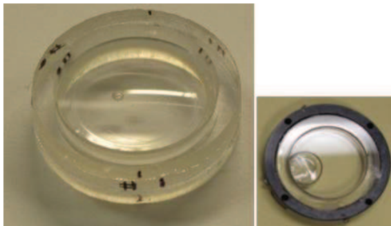
Figure 2.6: Air bubble inside a strong negative lenscore
