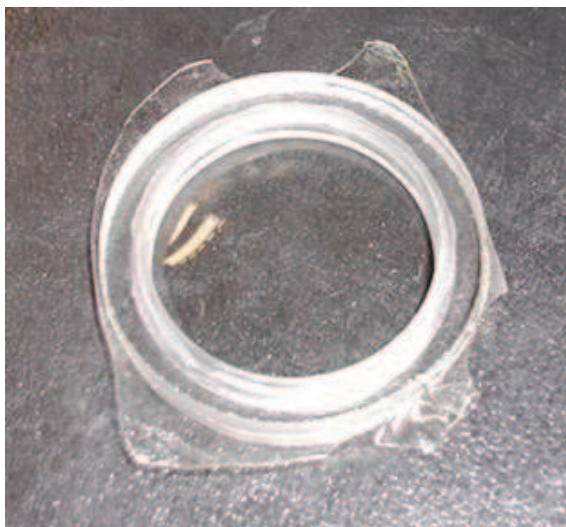
Figure 2.12: Thiol-ene membrane bonded un-stretched to glass using a heat catalyst adhesive
