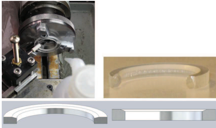
Figure 2.28: (Top) Straight bevel made on bench top lathe with cross section of result on glass ring. (Bottom) CAD of bevel.
