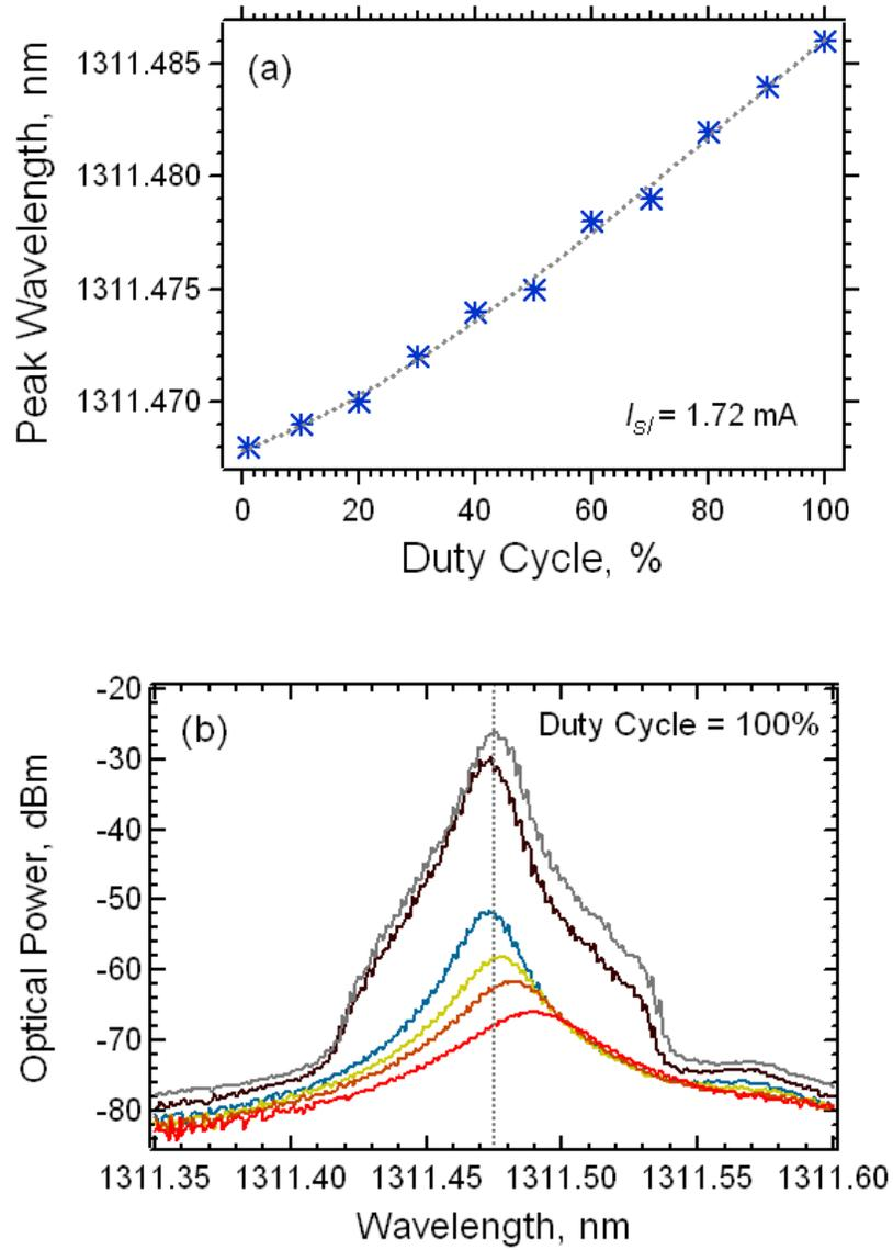
Figure 40. Quantum-dot laser: (a) Peak modal wavelength as a function of duty cycle. The pulse width was  $20\mu\text{s}$ . (b) Optical power response for subthreshold bias currents at 100% duty cycle. The bias currents correspond to 1.1 mA (red), 1.3 mA, 1.5 mA, 1.7 mA, 1.9 mA, and 2.0 mA (gray).
