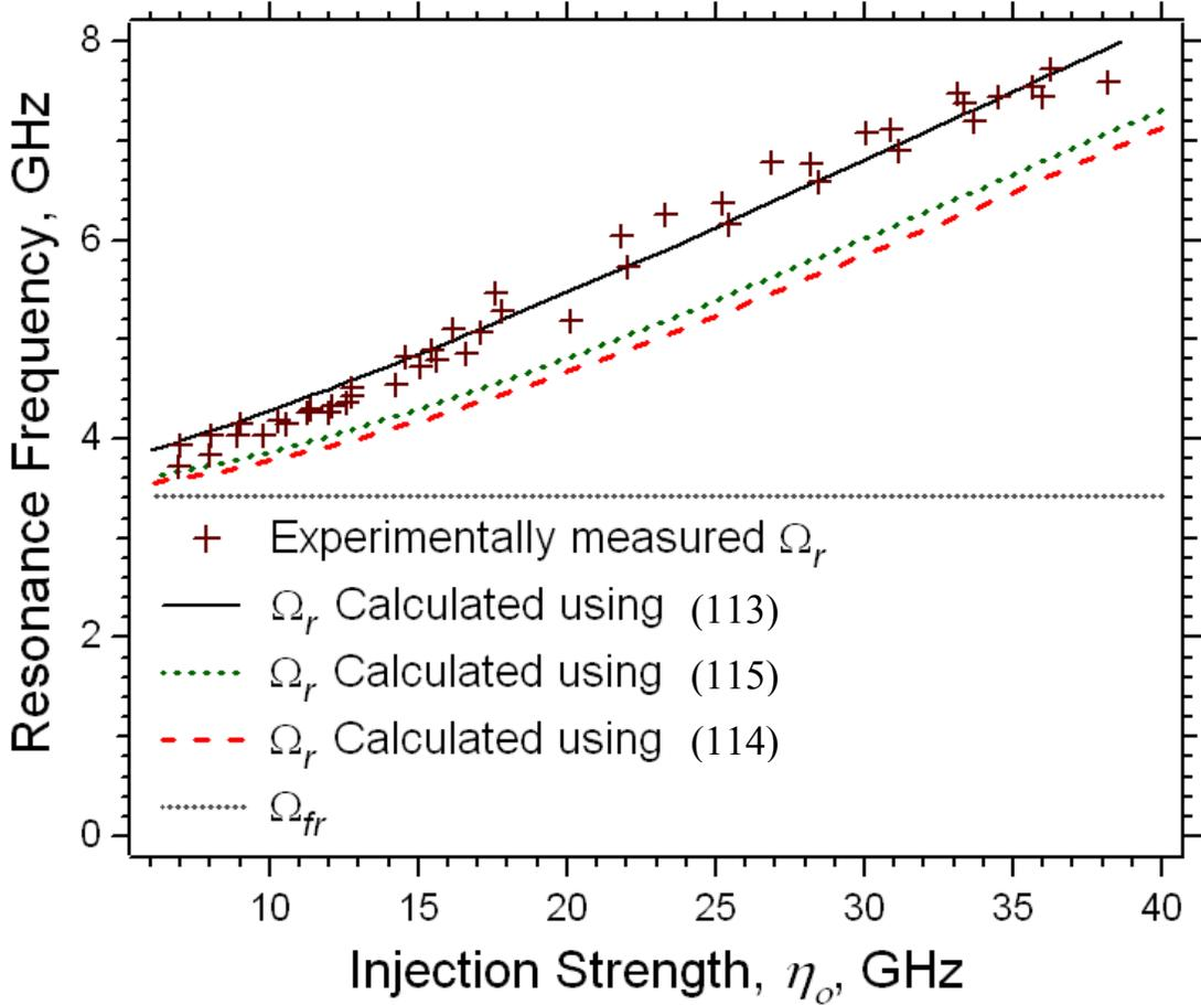
Figure 69. Measured and calculated period-one resonance frequency as a function of the injection strength for the quantum-dash slave laser at a bias current of 70 mA and zero-detuning. The resonance frequency was measured using the spectral sidebands as depicted in Figure 68.
