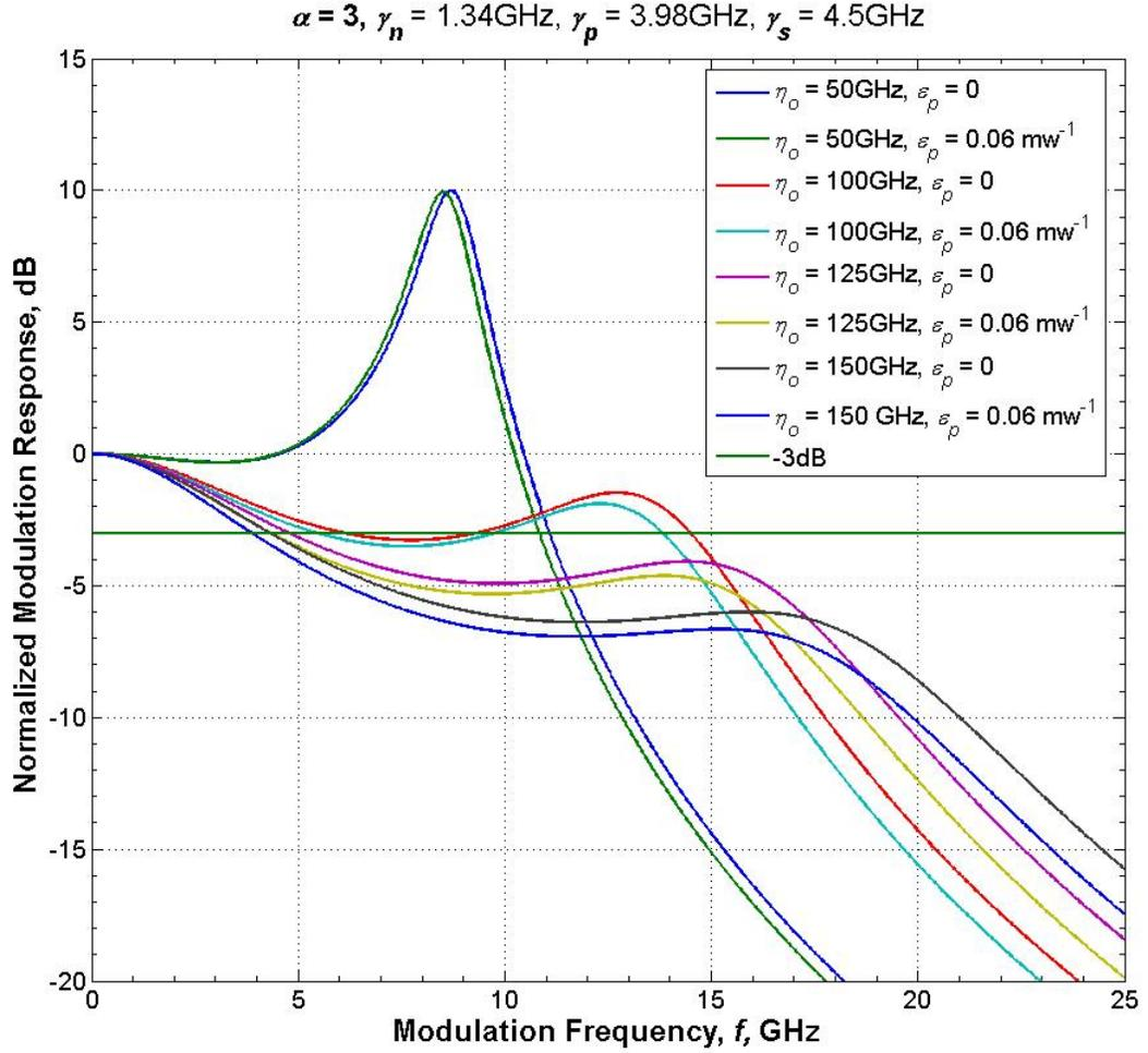
Figure 25. Microwave modulation response plotted both with and without the consideration of the gain compression coefficient shown in eqn. (74) on the differential and nonlinear carrier relation rate at zero-detuning;  $\alpha = 3$ . The free-running laser parameters are based on the quantum-dash laser biased at 70 mA, and the gain compression coefficient is  $0.06 \text{ mW}^{-1}$ .
