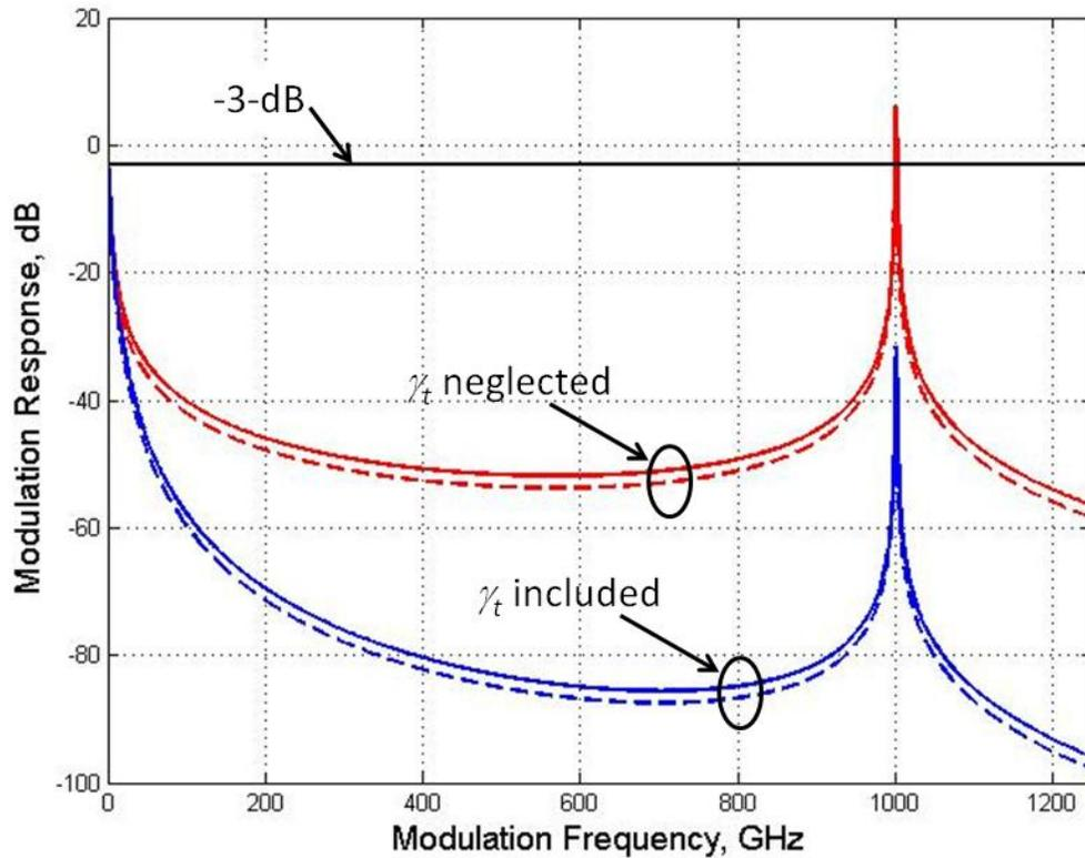
Figure 53. Theoretically simulated small-signal modulation response at the positive frequency detuning edge for a short cavity device ( $25 \mu\text{m}$ ) under strong injection ( $P_{inj} = 87.5 \text{ mW}$ ) to show a 1 THz resonance frequency. Cases where the inverse parasitic carrier transport time ( $\gamma_t$ ) is and is not considered are included. The dashed lines illustrate the impact of gain compression on the response.
