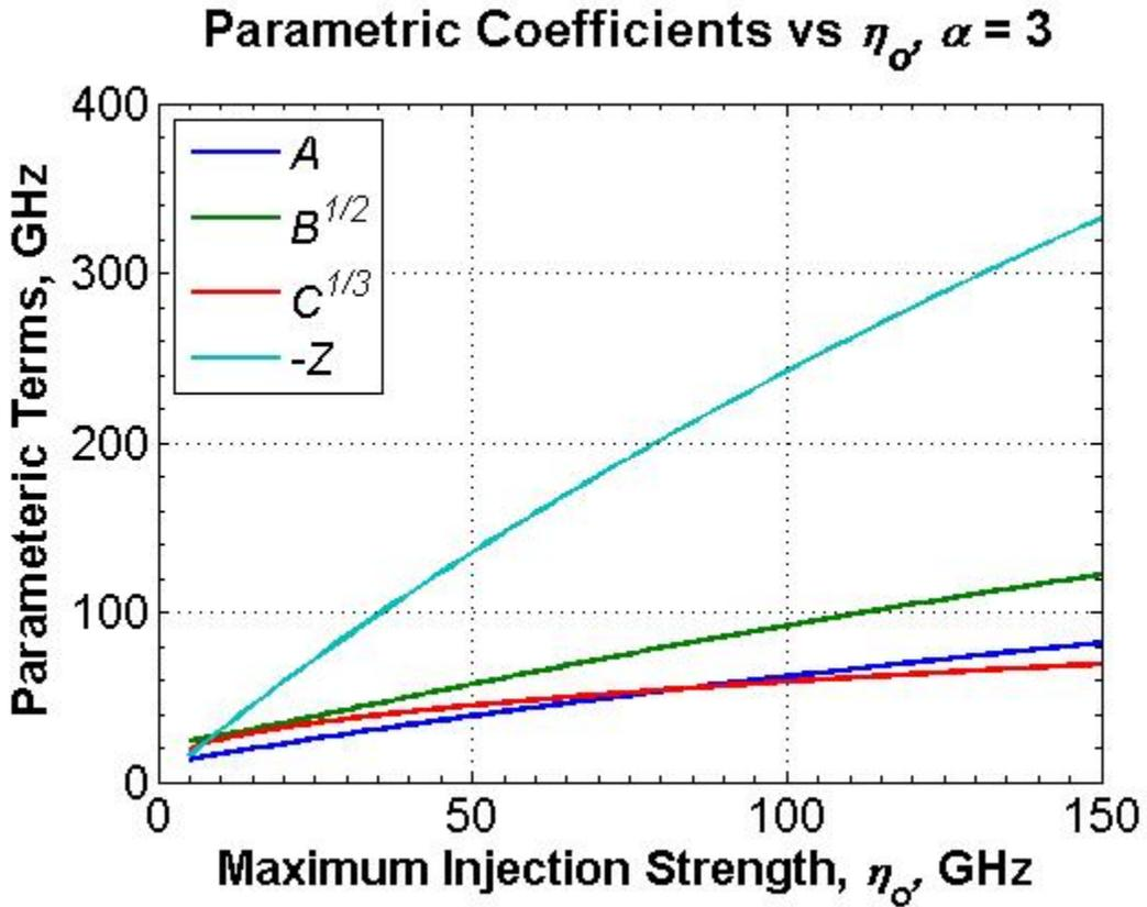
Figure 20.  $A$ ,  $B$ , and  $C$  coefficients as a function maximum injection strength at zero-detuning,  $\alpha = 3$ . Notice that the resonance frequency driving term,  $B^{1/2}$ , remains larger than the damping rate driving term,  $A$ . The free-running laser parameters are based on the quantum-dash laser biased at 70 mA ( $\gamma_n = 1.34$  GHz,  $\gamma_p = 3.98$  GHz,  $\gamma_s = 4.5$  GHz,  $\gamma_c = 333.3$  GHz).
