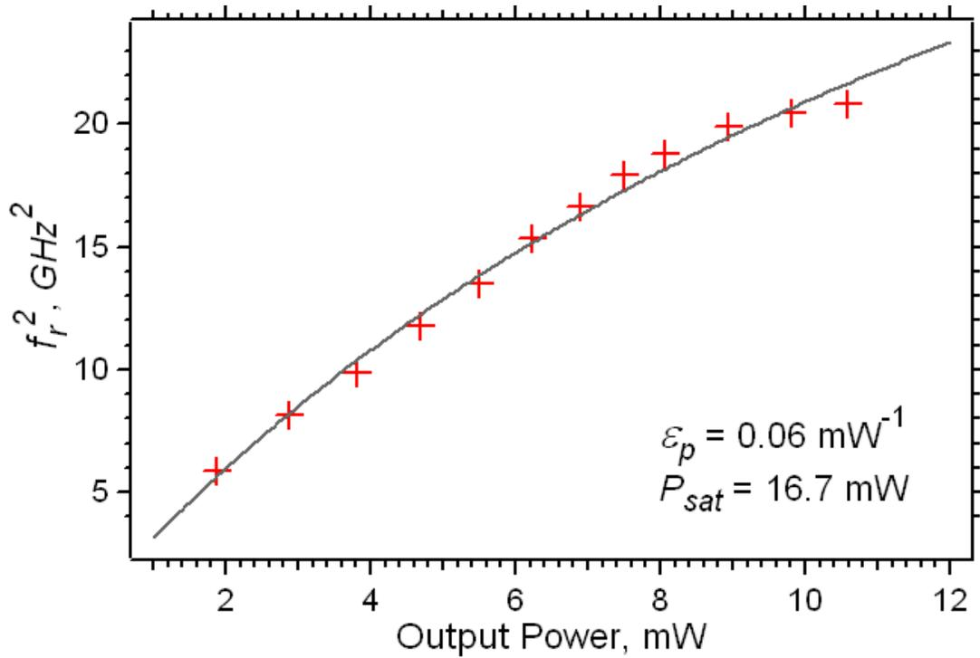
Figure 48. Quantum-dot laser free-running relaxation oscillation ( $f_r^2$ ) as a function of the total output power ( $P_{out}$ , both laser facets). The dotted line is a least squares linear fit using expression (93).
