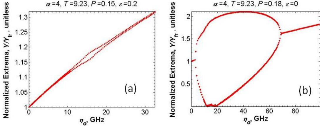
Figure 72. Bifurcation diagram for a linewidth enhancement parameter of 5 and relaxation rates based on a 5 mA bias current for the quantum-dot laser. (a) includes and (b) ignores the nonlinear carrier relaxation rate in the rate equations.
