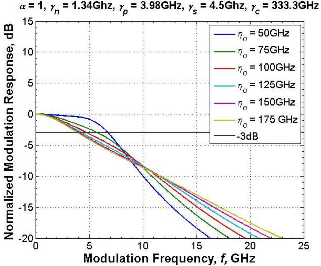
Figure 19. Modulation response as a function of maximum injection strength at zero-detuning,  $\alpha = 1$ . Compared with Figure 18, the response is more strongly damped. The free-running laser parameters are based on the quantum-dash laser biased at 70 mA.
