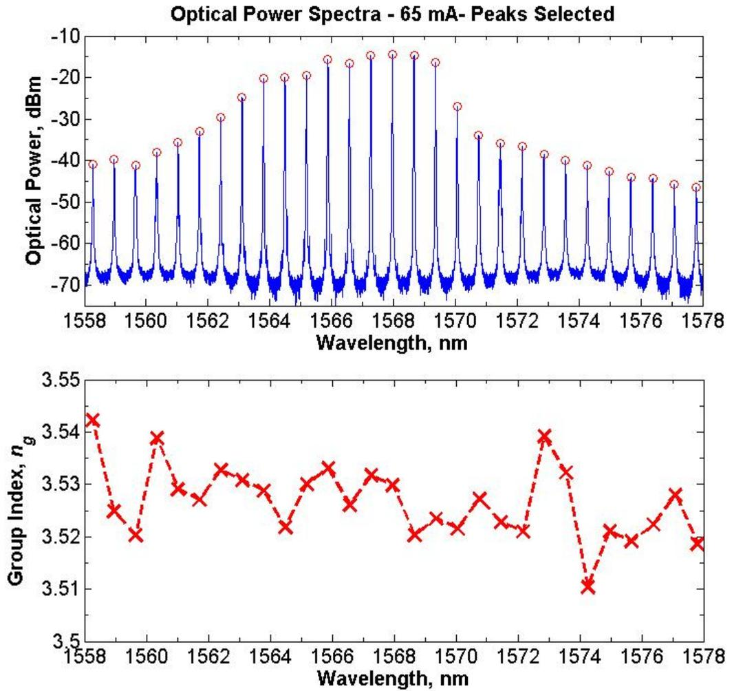
Figure 45. Group index of the active region as a function of Fabry-Perot mode at a bias current of 65 mA. The free-spectral range ( $\Delta\lambda$ ) was averaged between each two adjacent modes, and calculated using  $n_g = \lambda^2/(2L\Delta\lambda)$ .
