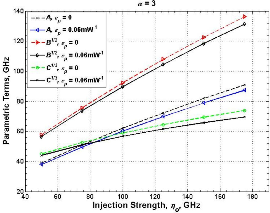
Figure 26.  $A$ ,  $B$ , and  $C$  parametric terms plotted both with and without the consideration of the gain compression effect on the differential and nonlinear carrier relation rates plotted as a function of maximum injection strength at zero-detuning;  $\alpha = 3$ . The free-running laser parameters are based on the quantum-dash laser biased at 70 mA, and the gain compression coefficient is  $0.06 \text{ mW}^{-1}$ .
