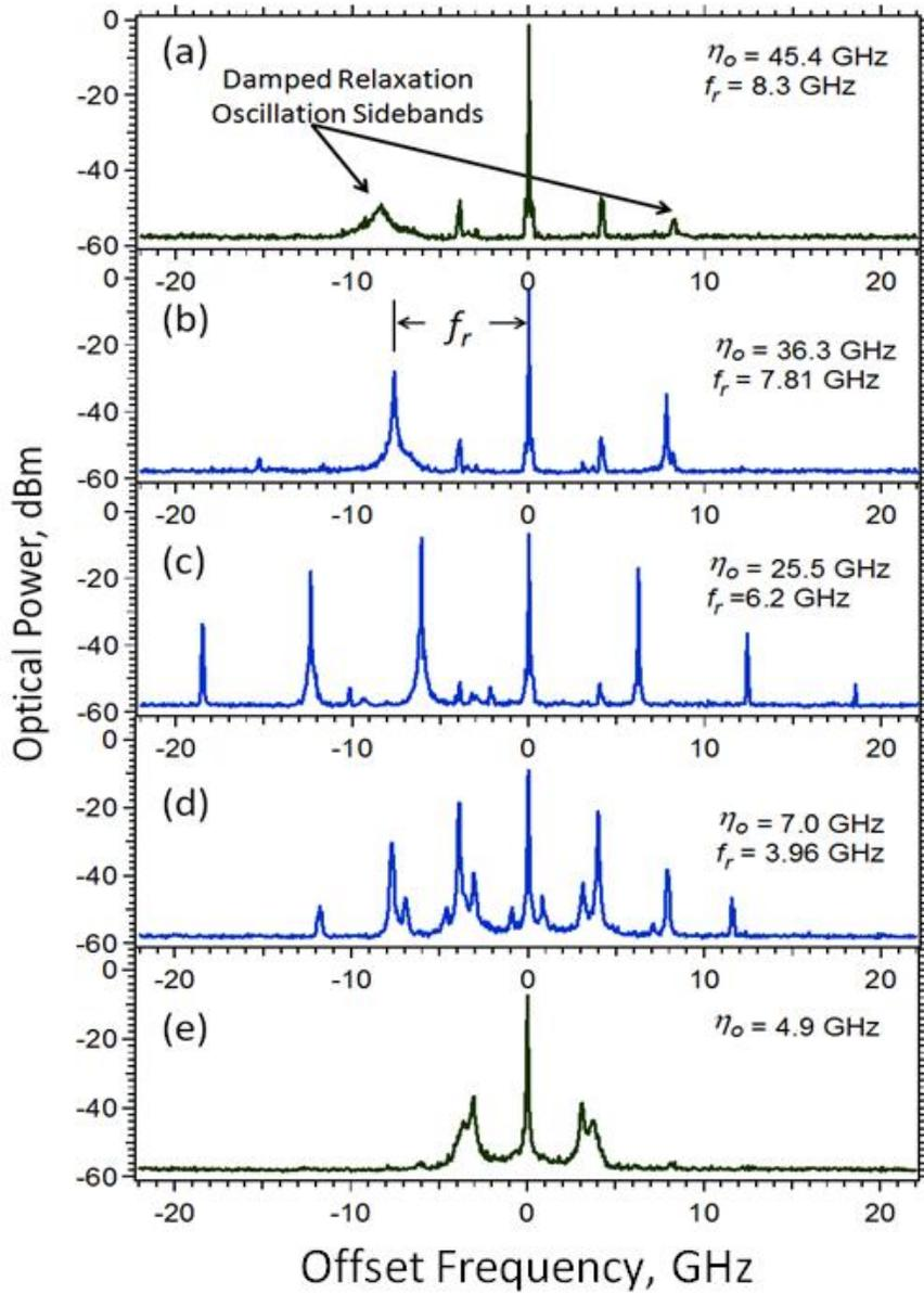
Figure 68. Optical spectra of the optically injected quantum-dash slave laser under a bias of 70 mA and zero-detuning showing the increase in resonance frequency with injection strength.  $f_r$  is the measured resonance frequency value. The spectra shown in blue are within the period-one operational region. The oscillations below -40 dBm are a result of residual feedback in the experimental setup.
