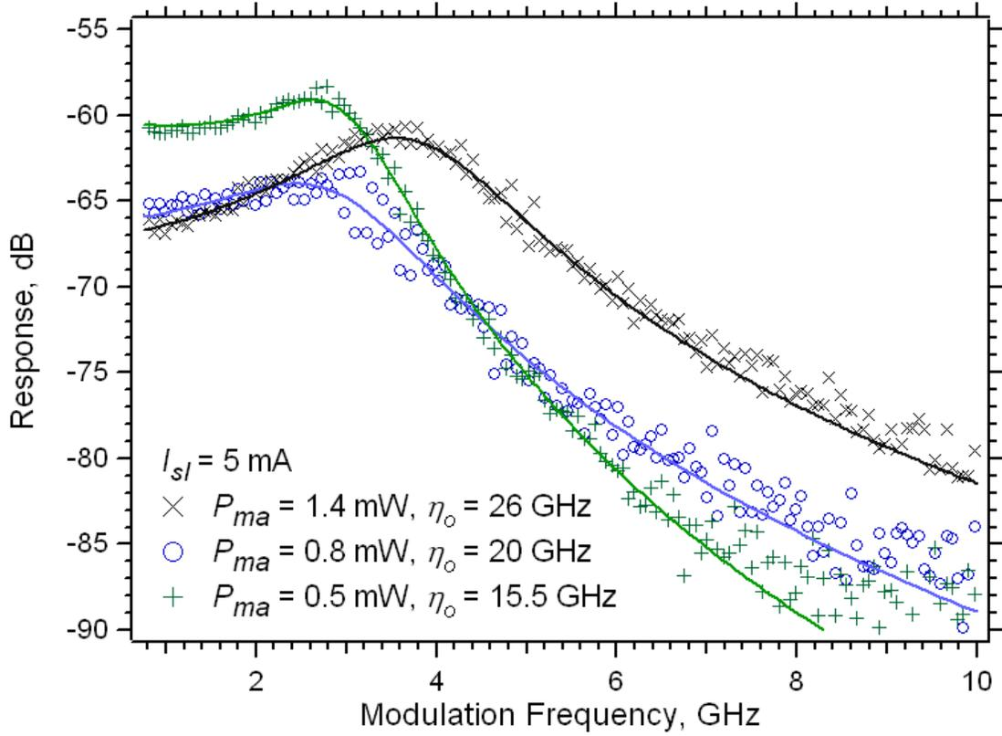
Figure 78. Small-signal modulation response at zero-detuning showing the least-square fitting results.
