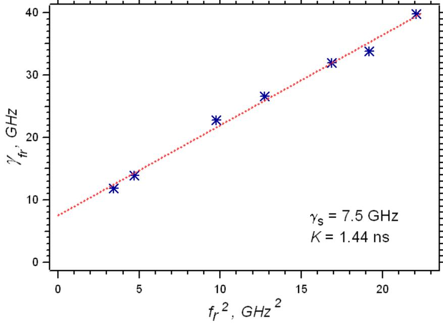
Figure 38. Free-running damping rate ( $\gamma_{fr}$ ) as a function of the relaxation oscillation frequency squared ( $f_{fr}^2$ ). The dotted red line is a least-squares linear fit to the data points, which is extrapolated to determine the spontaneous carrier relaxation rate,  $\gamma_s$ .
