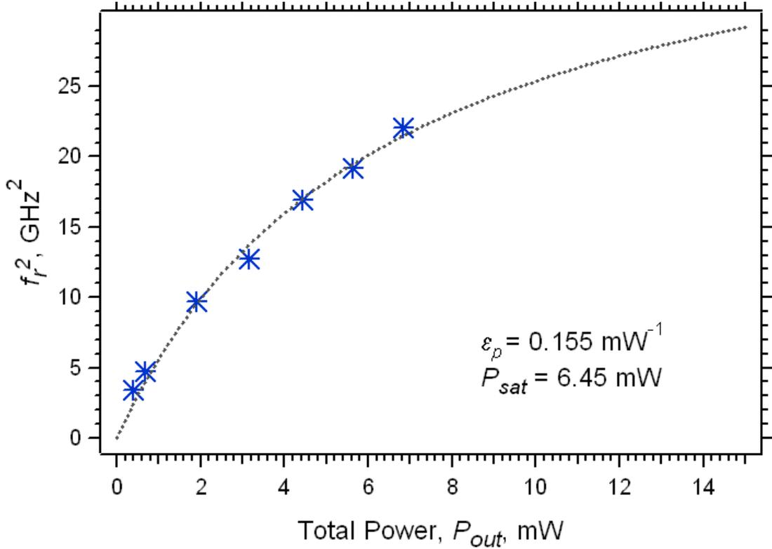
Figure 39. Quantum-dot laser free-running relaxation oscillation ( $f_r^2$ ) as a function of the total output power ( $P_{out}$ ). The dotted line is a least squares linear fit using expression (93), where the gain compression coefficient is found to be  $0.155 \text{ mW}^{-1}$ . In each plot, the experimental values (blue asterisks) correspond to laser bias currents of 3.8, 5, 10, 15, 20, 25, and 30 mA.
