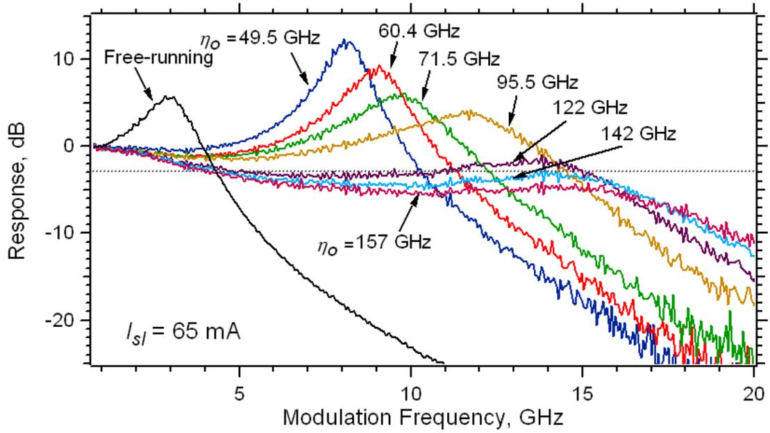
Figure 54. Normalized microwave modulation response under zero-detuning for increased injection strengths; slave bias is 65 mA.
