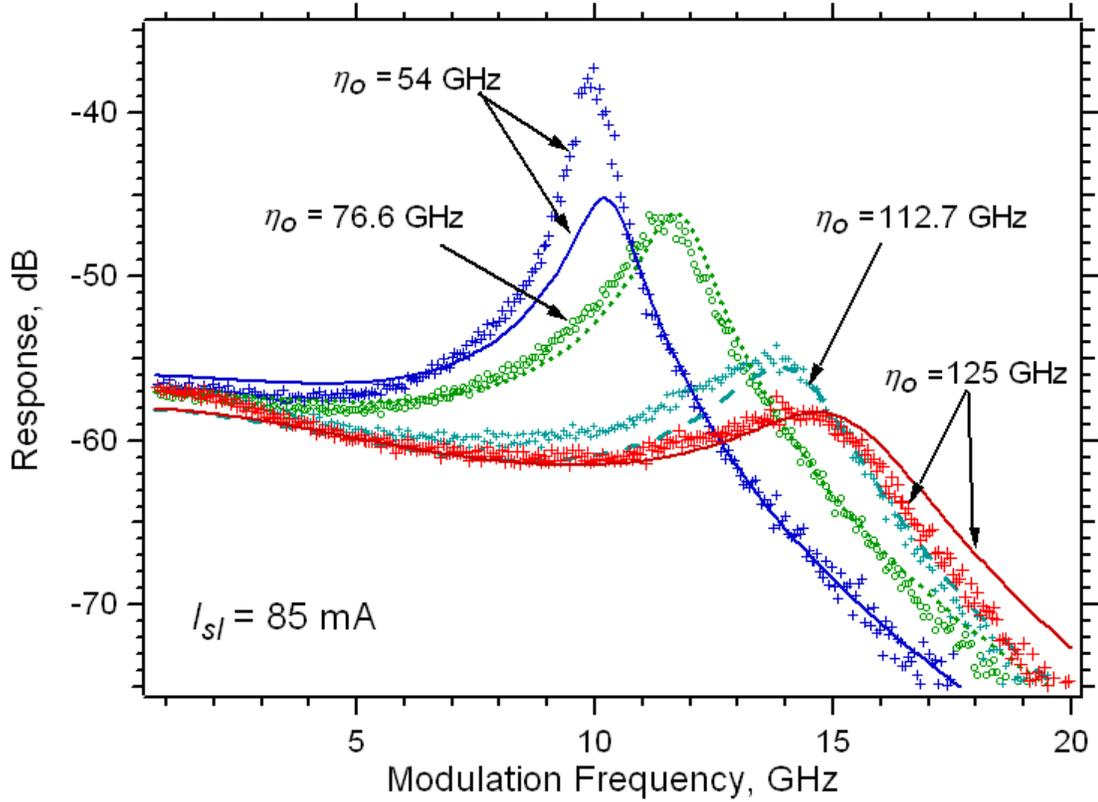
Figure 60. Least-square-fit modulation response under zero-detuning for increased injection strengths; slave bias is 85 mA. The linewidth enhancement parameter is restricted to:  $5 < \alpha < 8$ . Markers indicate experimental data; the fitting results are given by the solid and dashed lines.
