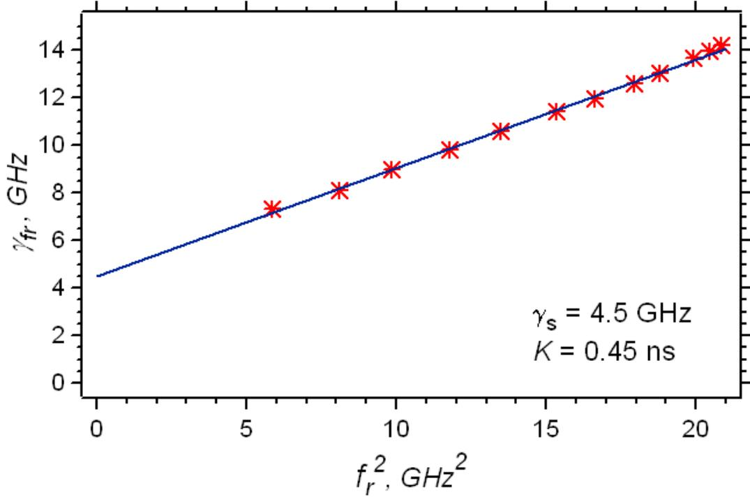
Figure 47. Free-running damping rate ( $\gamma_{fr}$ ) as a function of the relaxation oscillation frequency squared ( $f_r^2$ ). The blue line is a least squares linear fit to the data points, which is then extrapolated to determine the spontaneous carrier relaxation rate,  $\gamma_s$ .
