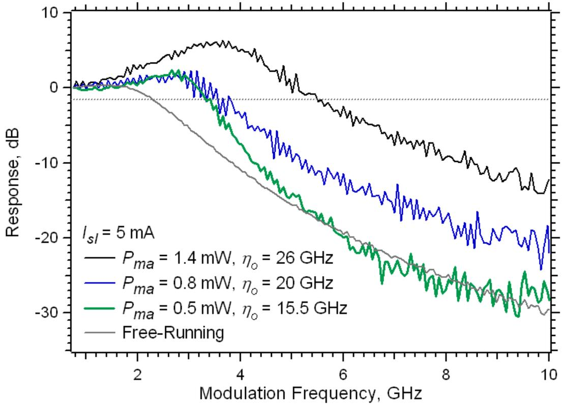
Figure 77. Normalized small-signal modulation response at zero-detuning.
