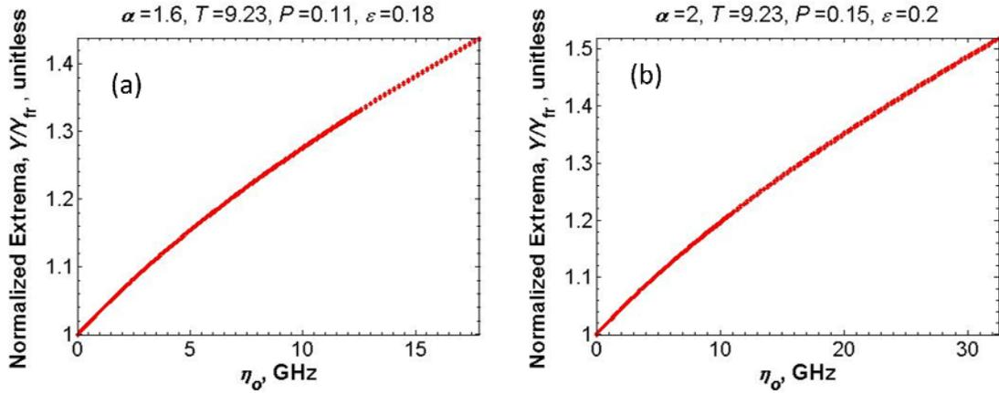
Figure 71. Bifurcation diagrams simulating the response under zero-detuning. The two cases correspond to respective  $P$ ,  $T$ , and  $\alpha$ -factor values for 3.8 mA (2X  $I_{th}$ ), and 5 mA (2.6X  $I_{th}$ ) bias conditions and illustrate the stability of the quantum-dot slave laser's operational behavior.
