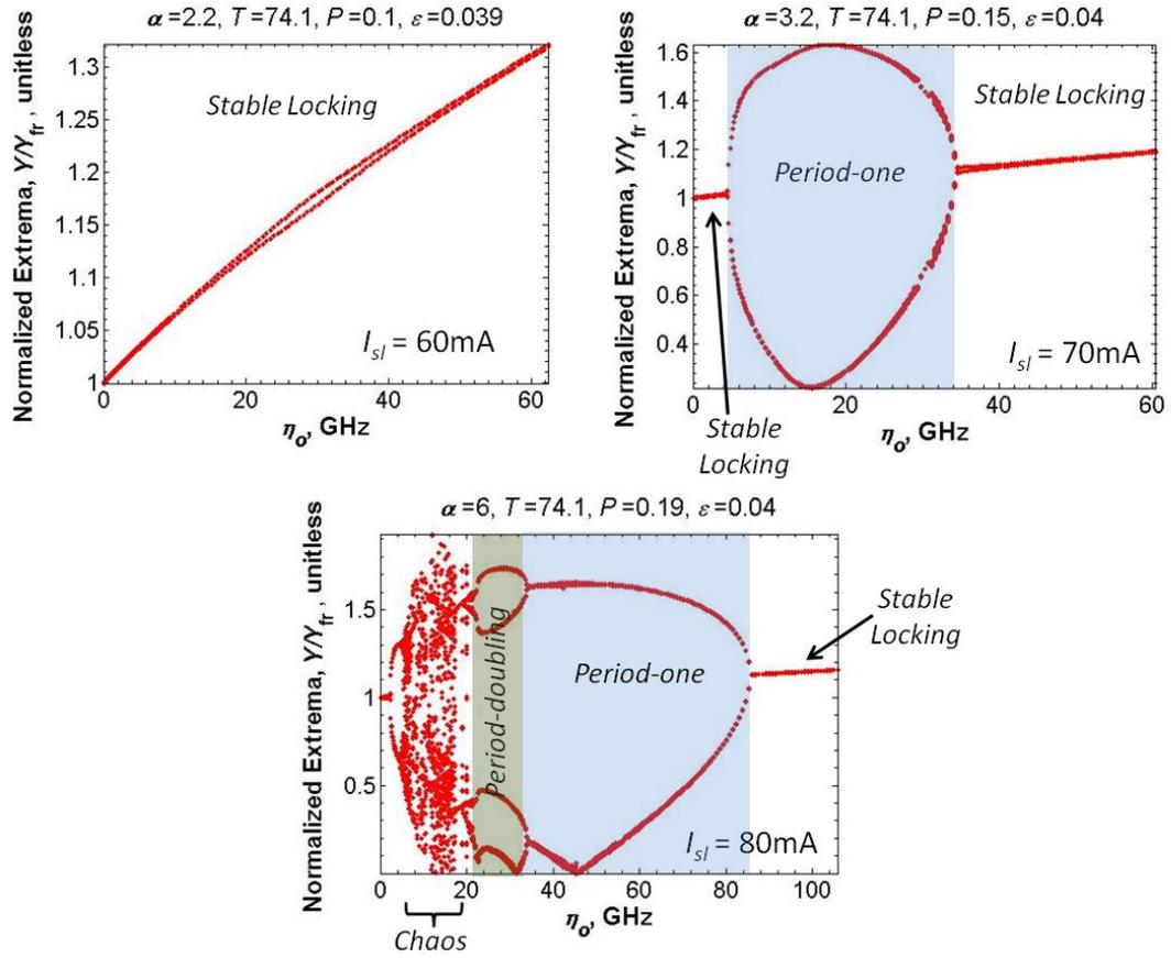
Figure 28. Bifurcation diagrams showing theoretical solutions to the normalized rate equations in (88) - (90) for zero-detuning conditions. The four cases correspond to respective P, T, and  $\alpha$ -factor values for 60, 70, and 80 mA slave bias conditions of the quantum-dash slave laser.
