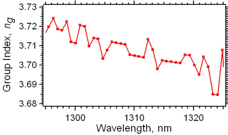
Figure 36. Group index of the active region as a function of Fabry-Perot mode at a bias current of 5 mA. The free-spectral range ( $\Delta\lambda$ ) was averaged between each two adjacent modes, and calculated using  $n_g = \lambda^2/(2L\Delta\lambda)$ .
