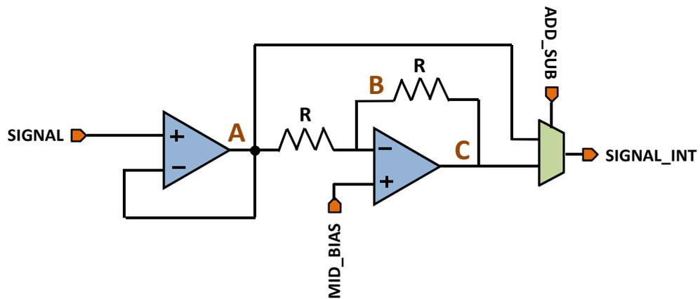
Figure 3.2: Analog optional inverter with buffer stage
