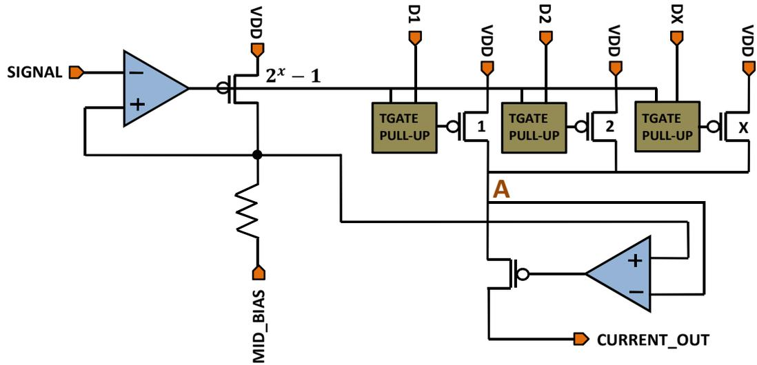
Figure 5.12: Push section of the current bias and current multiplier
