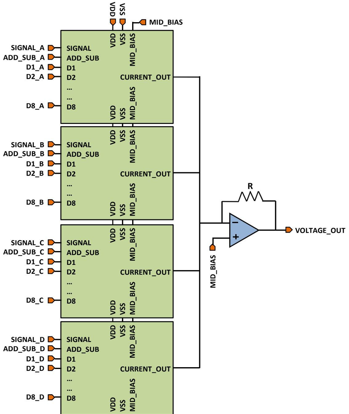
Figure 7.2: Full analog signal multiply and accumulate circuit.
