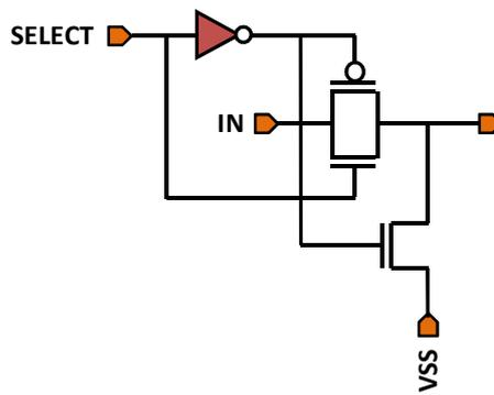
Figure 5.7: Pass gate with integrated pull-down
