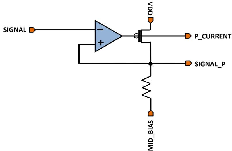
Figure 4.1: PMOS signal voltage to signal current converter
