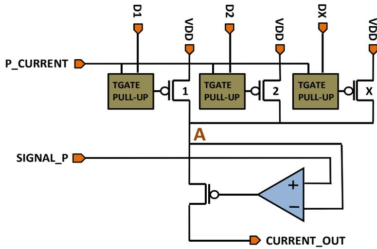
Figure 5.6: Push section of the current multiplier
