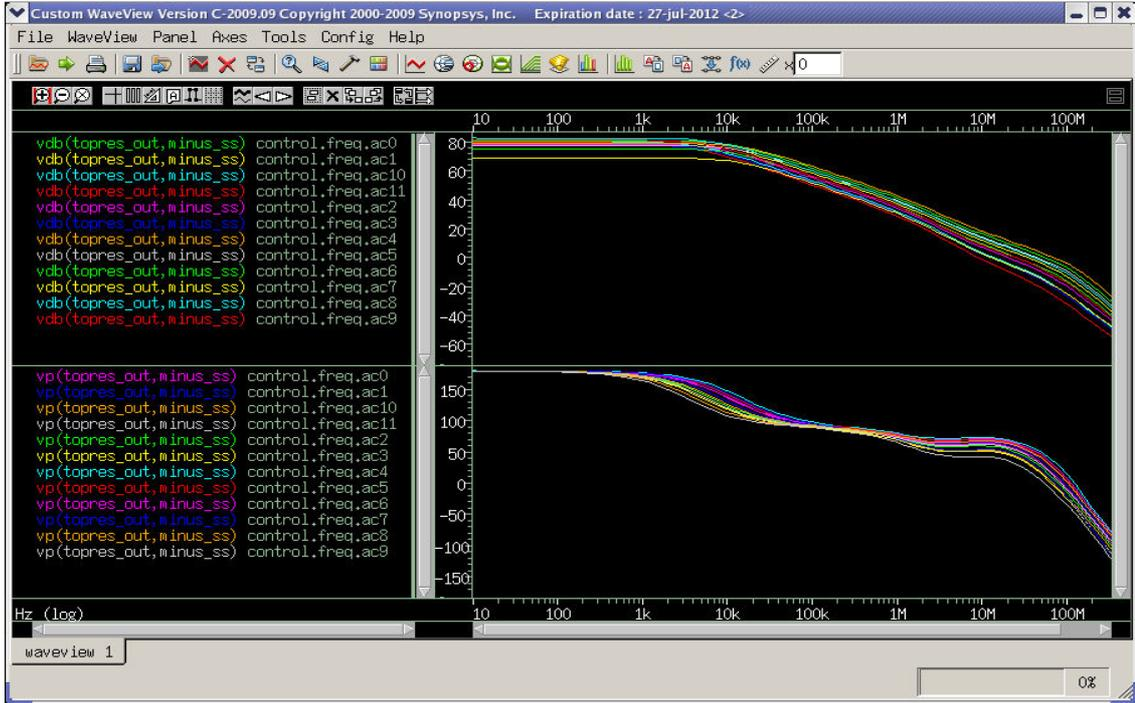
Figure 4.7: Wave forms of the PMOS current bias frequency analysis
