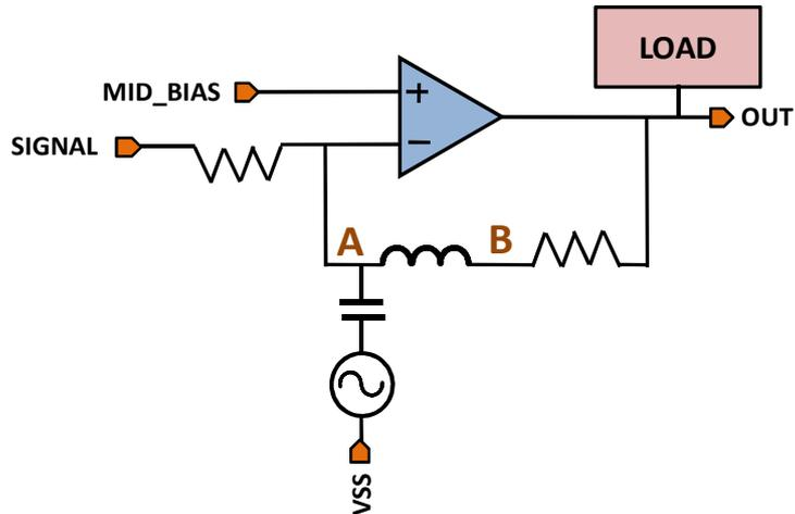
Figure 3.4: Stability analysis setup for the analog inverter
