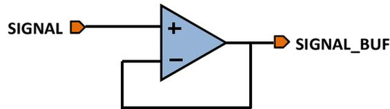
**Figure 2.2: Analog operational amplifier buffer**
