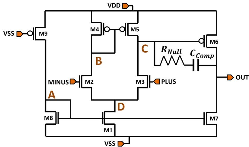
Figure 2.1: Circuit diagram of an NMOS differential pair two stage operational amplifier
