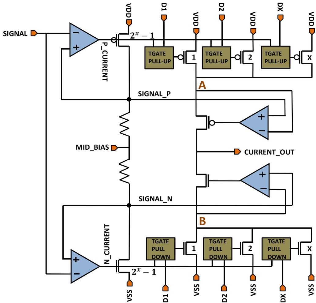
Figure 5.14: Full swing current bias and current multiplier
