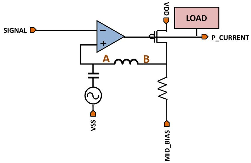
Figure 4.5: PMOS current bias stability analysis setup
