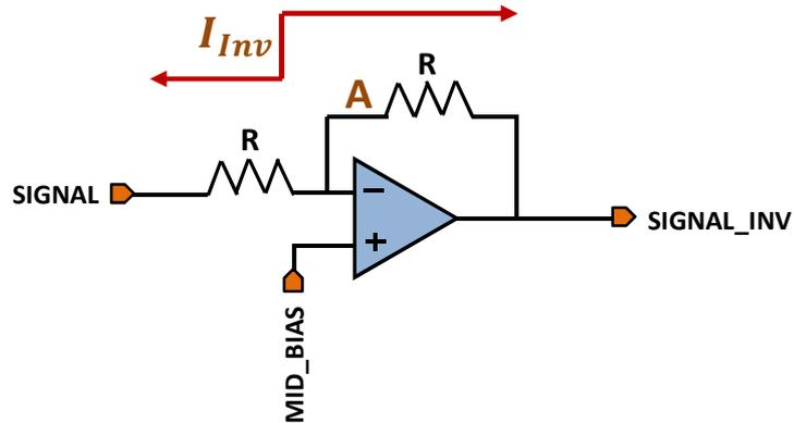
**Figure 3.1: Analog operational amplifier inverter**
