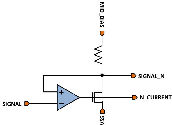
Figure 4.2: NMOS signal voltage to signal current converter
