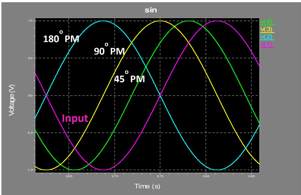
**Figure 2.5: Phase shifts for different phase margins (PM)**
