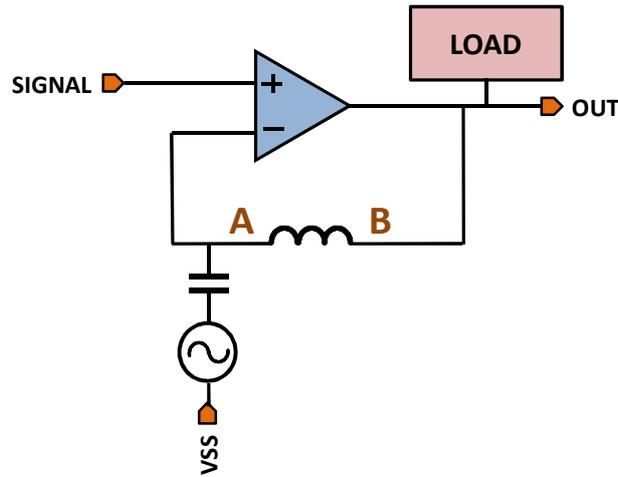
**Figure 2.4: Stability analysis setup for the analog buffer**
