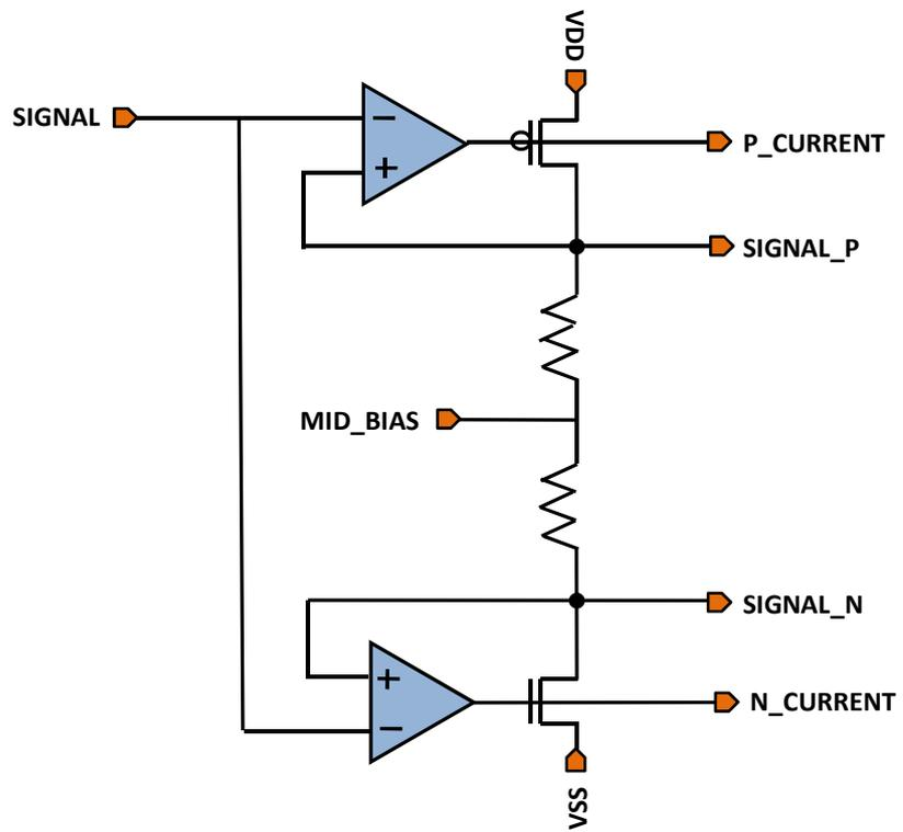
Figure 4.3: Full push/pull signal voltage to signal current converter
