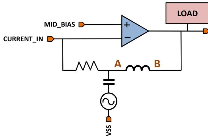
Figure 6.2: Stability analysis setup for the regulated current to voltage converter
