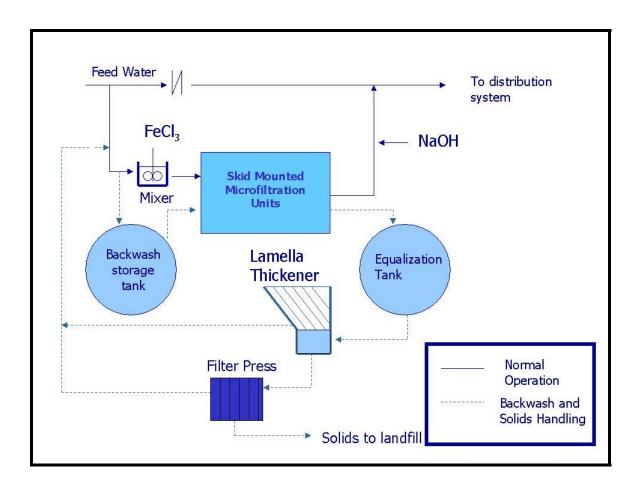
Figure 5: Coagulation/Microfiltration Treatment Process Diagram
