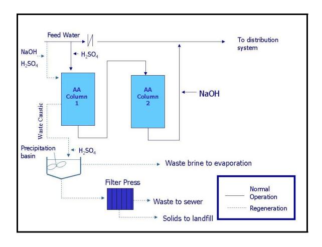
Figure 4: Activated Alumina Treatment Process Diagram
