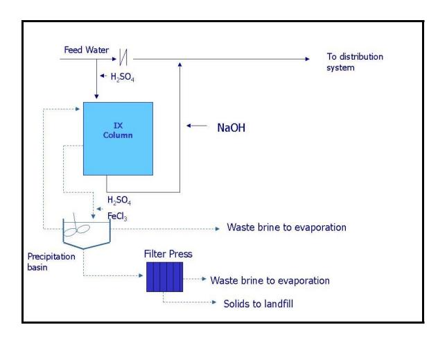
Figure 3: Ion Exchange Treatment Process Diagram
