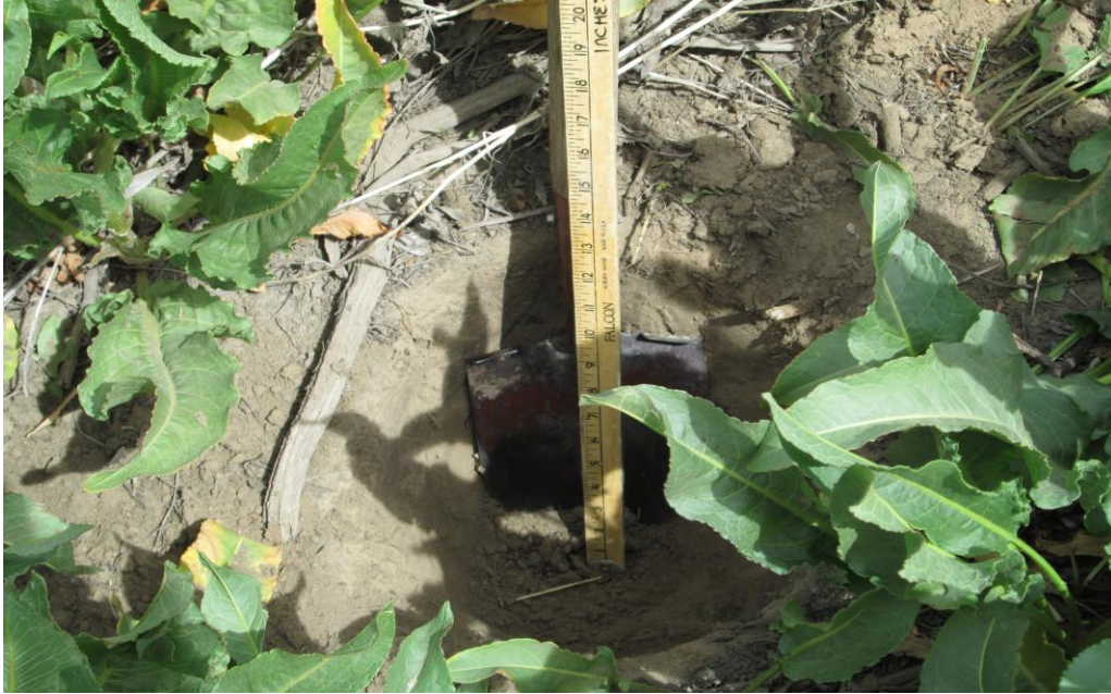
Figure 10: Typical excavated sample site, depth of hole is 12 inches
