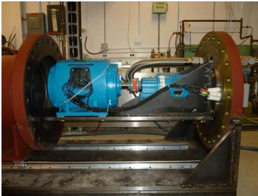
Figure 1.3: Photograph of the Roots Blower (Left) and Motor (Right) Mounted to a Plate Cantilevered of the End of the Pressure Vessel Flange Plate. The Other End of the Pressure Vessel Slides Back and Forth Over the Motor and Blower on Rails Bolted to the Skid Plate
