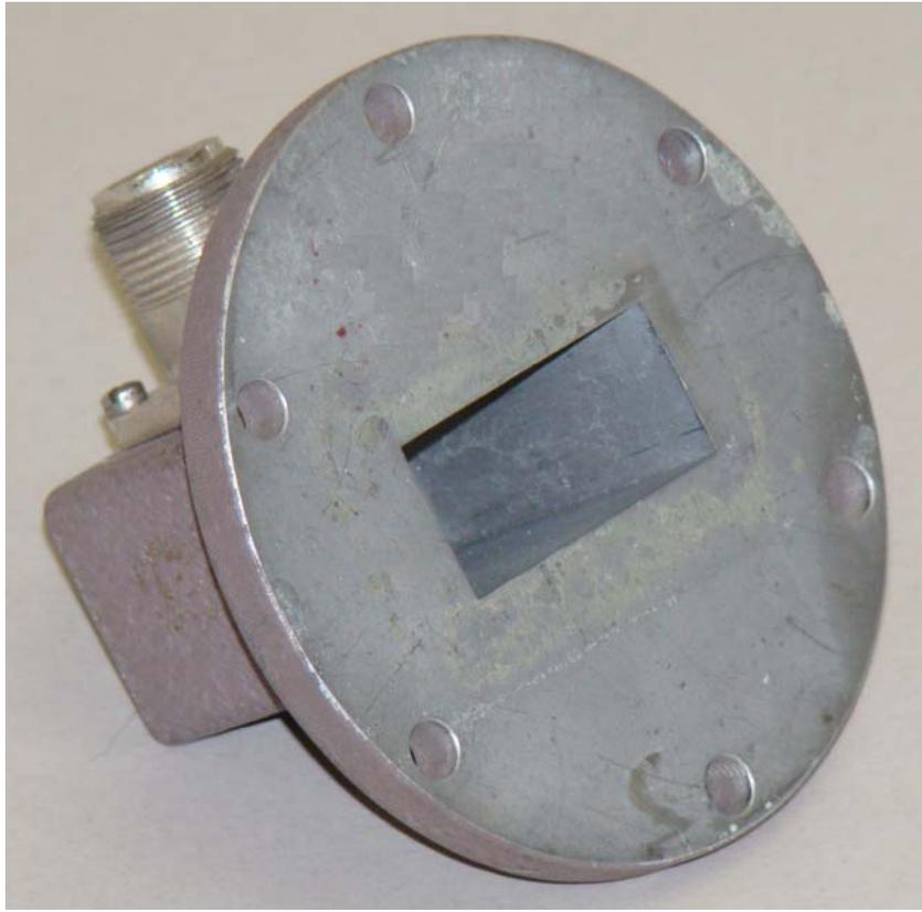
**Figure 3.12.- Waveguide-to-SMA transition.**
