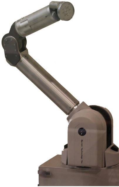
Figure 3.2: Whole Arm Manipulator by Barrett Technologies
