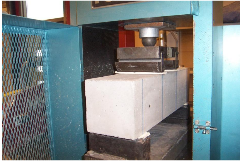
Figure 3.8 – Modulus of rupture testing
