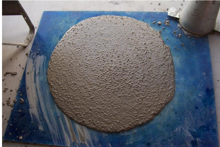
Figure 3.5 – Slump flow test
