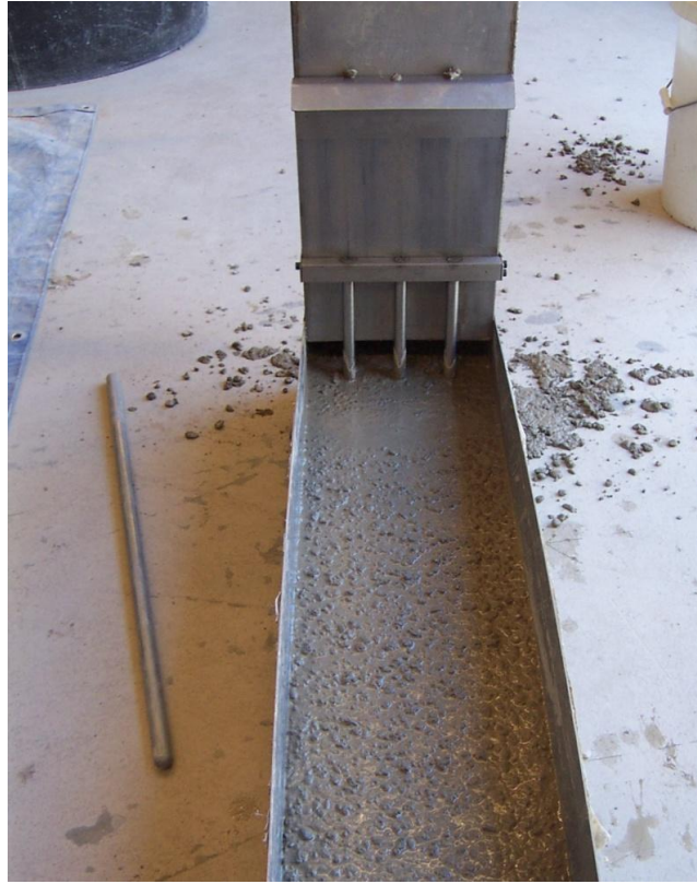
Figure 3.7 – L-Box test to determine SCC passing ability
