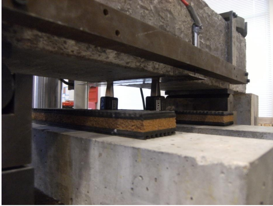
Figure 3.16 – Installation of clip gages
