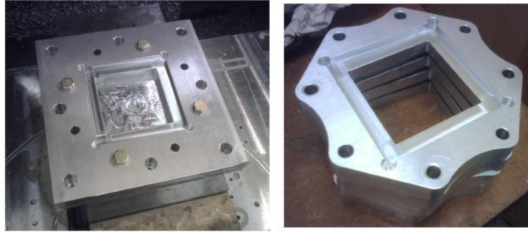
Figure 3.10: (left) Aluminum plate used to fabricate shock tube with stock material bolted to a CNC machine. (right) Completed flanges, fabricated in the UNM student machine shop.
