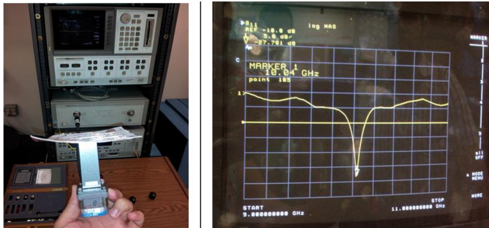
Figure 50: Fabrication and measurement of the 10GHz antenna
