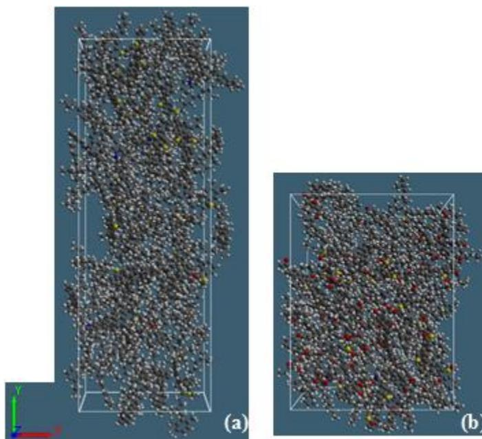
**Figure 5.7** Configurations of asphalt systems before (a) and after (b) oxidation under tensile stress rate of 284 GPa sec<sup>-1</sup>
