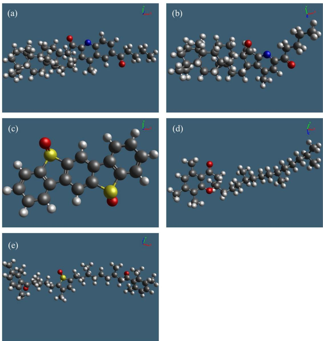
**Figure 3.7** Resin fraction after oxidative aging: (a) oxidized quinolinohopane,  $C_{40}H_{55}NO_2$ , (b) oxidized pyridinohopane,  $C_{36}H_{53}NO_2$ , (c) oxidized benzobisbenzothiophene,  $C_{18}H_{10}S_2O_2$ , (d) oxidized trimethylbenzene-oxane,  $C_{29}H_{48}O_2$ , and (e) oxidized thio-isorenieratane,  $C_{40}H_{56}SO_3$
