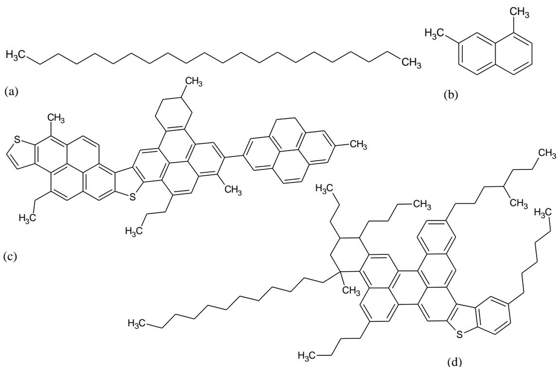
**Figure 2.8** Preliminary asphalt component models of Zhang and Greenfield's (2007a) study: (a) *n*-docosane ( $n\text{-C}_{22}\text{H}_{46}$ ), (b) 1,7-dimethylnaphthalene, (c) asphaltene 1, and (d) asphaltene 2
