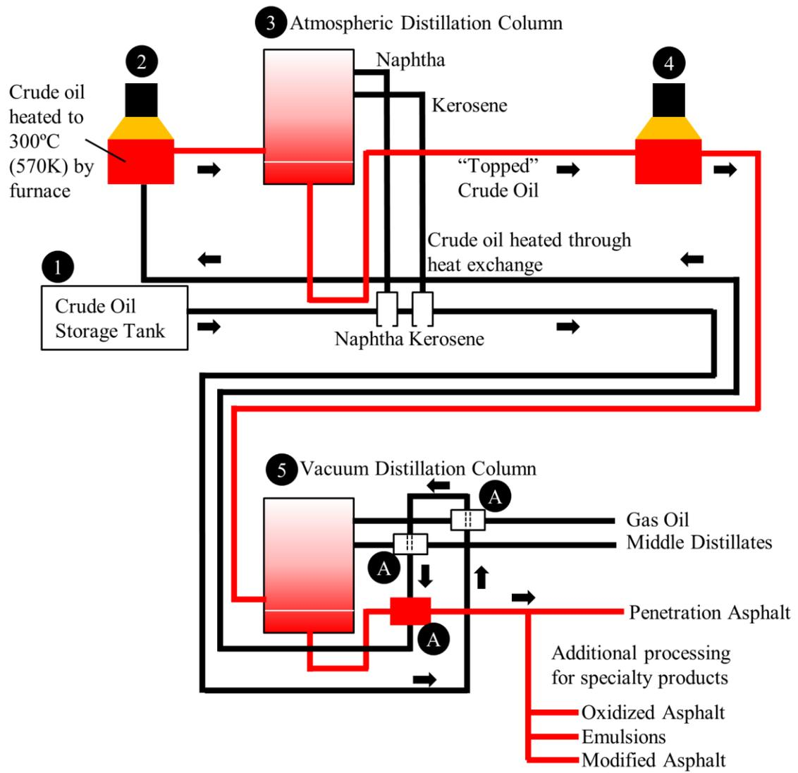
**Figure 2.1** Typical distillation process of asphalt (Lesueur 2009)
