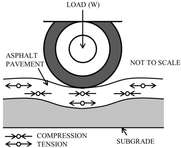
**Figure 1.1** Effects of traffic loading on AC layer
