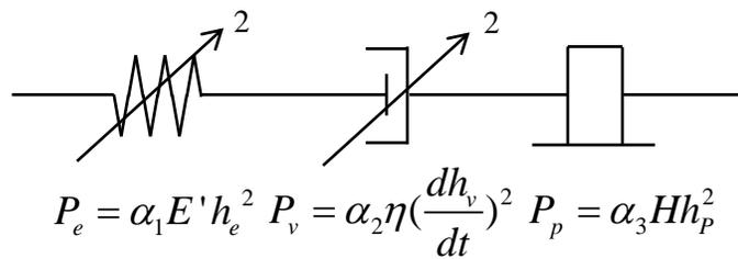
**Figure 7.10** Spring-Dashpot-Rigid (SDR) element model
