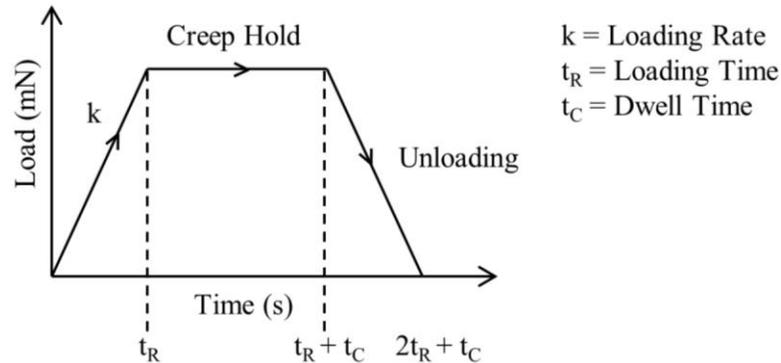
**Figure 7.11** Schematic of a trapezoidal indentation load
