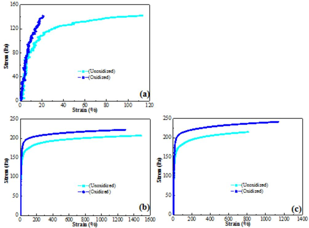
**Figure 5.10** Stress-strain curves for unoxidized and oxidized asphalts under different tensile stress rates: (a) 284 GPa sec<sup>-1</sup>, (b) 709 GPa sec<sup>-1</sup>, and (c) 993 GPa sec<sup>-1</sup>
