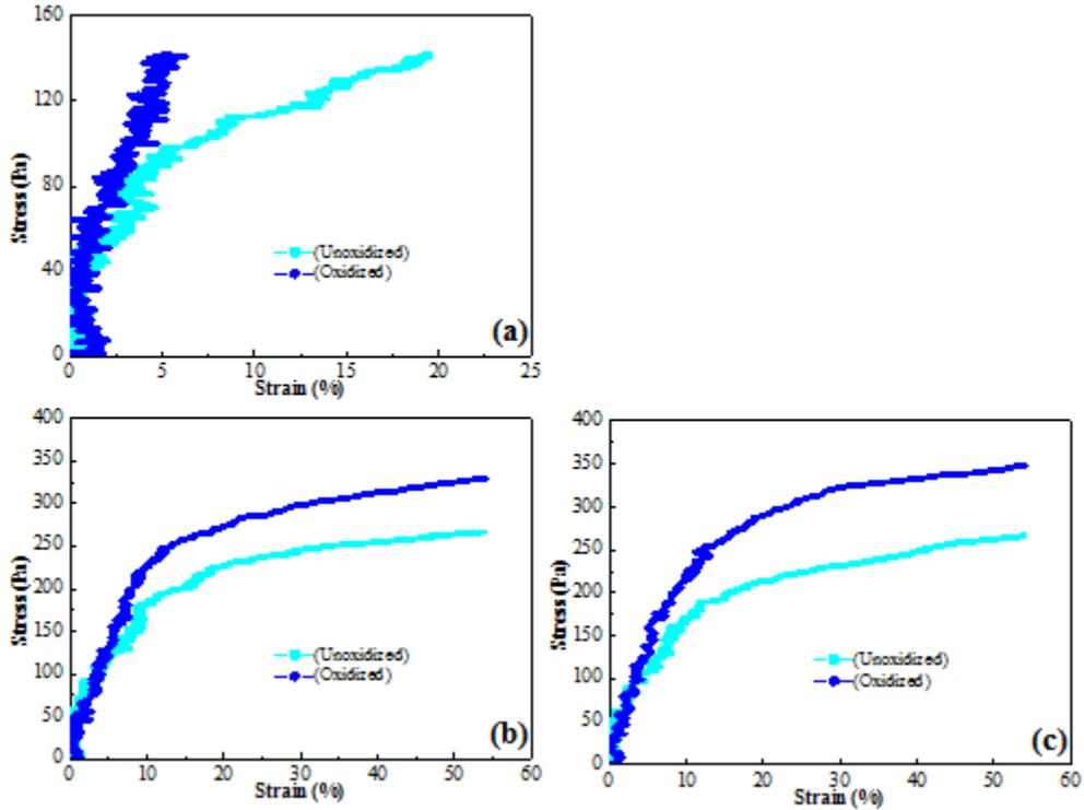
**Figure 5.5** Stress-strain curves for unoxidized and oxidized asphalts under different compressive stress rates: (a) 284 GPa sec<sup>-1</sup>, (b) 709 GPa sec<sup>-1</sup>, and (c) 993 GPa sec<sup>-1</sup>
