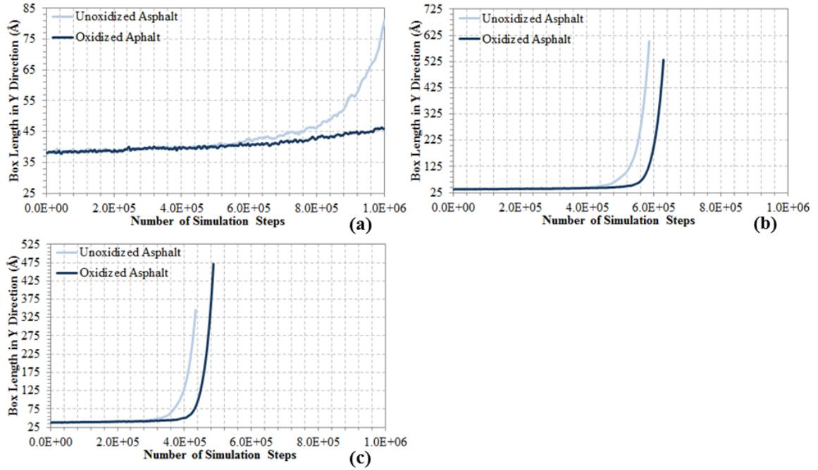
**Figure 5.9** Comparison of unoxidized and oxidized asphalts under different tensile stress rates: (a) 284 GPa sec<sup>-1</sup>, (b) 709 GPa sec<sup>-1</sup>, and (c) 993 GPa sec<sup>-1</sup>
