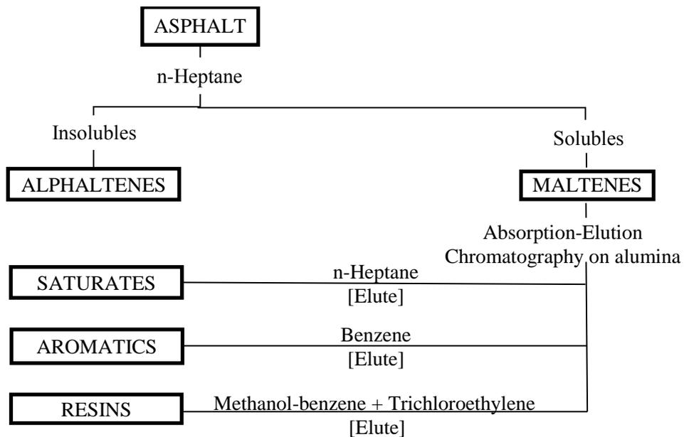
**Figure 2.2** Schematic of Corbett's (1969) asphalt separation method
