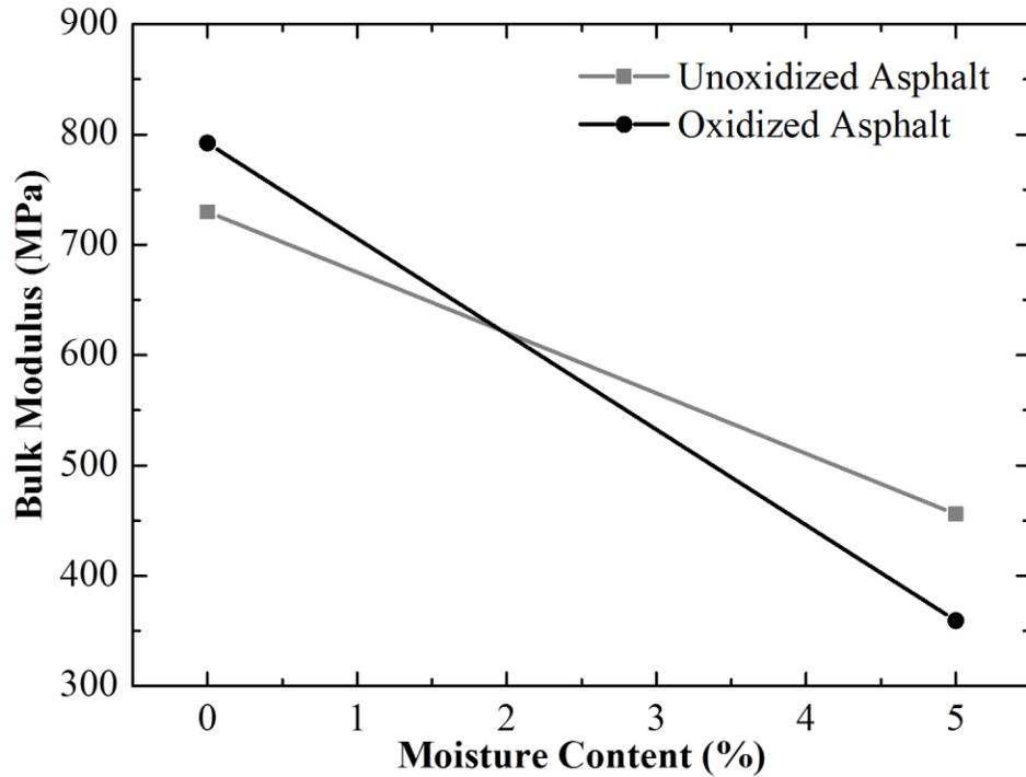
**Figure 7.3** Bulk modulus changes of unoxidized and oxidized asphalts under different moisture contents
