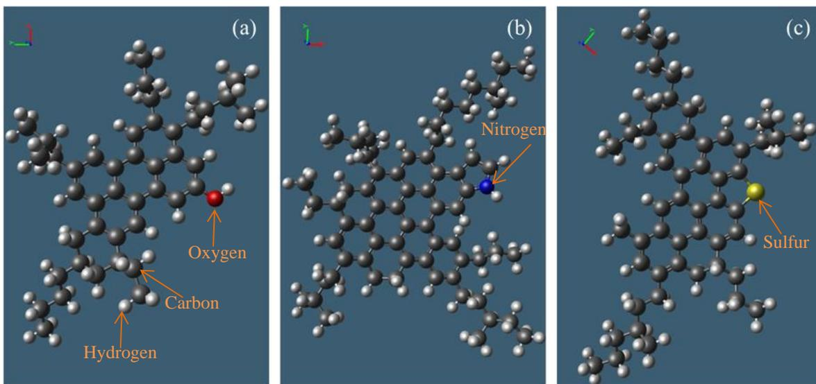
**Figure 3.1** Molecular structures of asphaltene fraction: (a) asphaltene-phenol,  $C_{42}H_{54}O$ , (b) asphaltene-pyrrole,  $C_{66}H_{81}N$ , and (c) asphaltene-thiophene,  $C_{51}H_{62}S$  (Li and Greenfield 2014)
