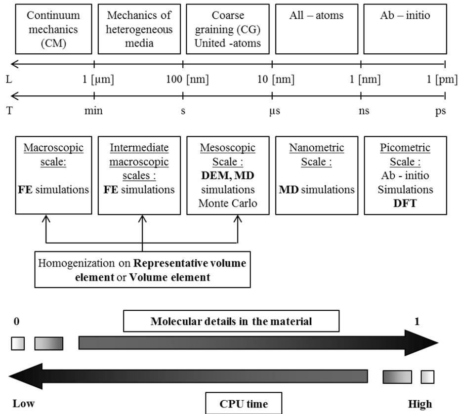
Figure 2.7 Schematic of Multi-Scale Modeling (Solar et al. 2012)
