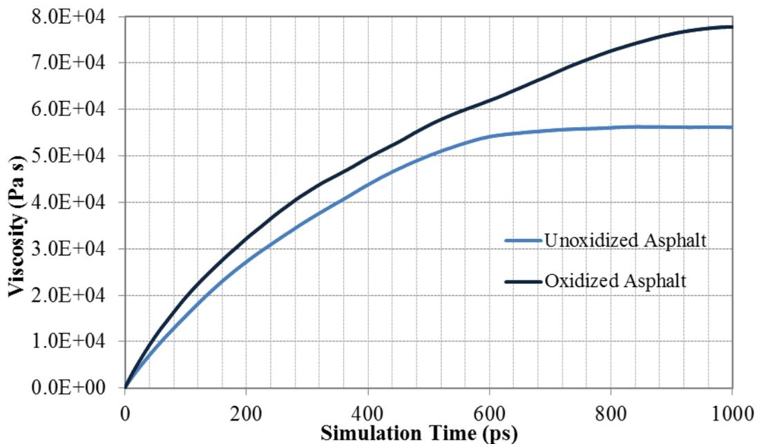
**Figure 4.6** Zero shear viscosity changes of asphalt before and after oxidative aging
