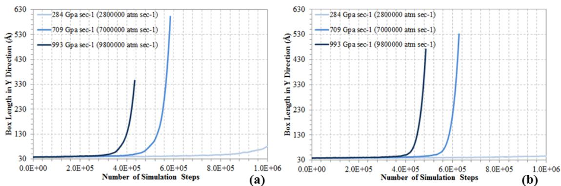
**Figure 5.6** Simulation results of unoxidized and oxidized asphalts under different tensile stress rates in Y direction with (a) unoxidized asphalt and (b) oxidized asphalt
