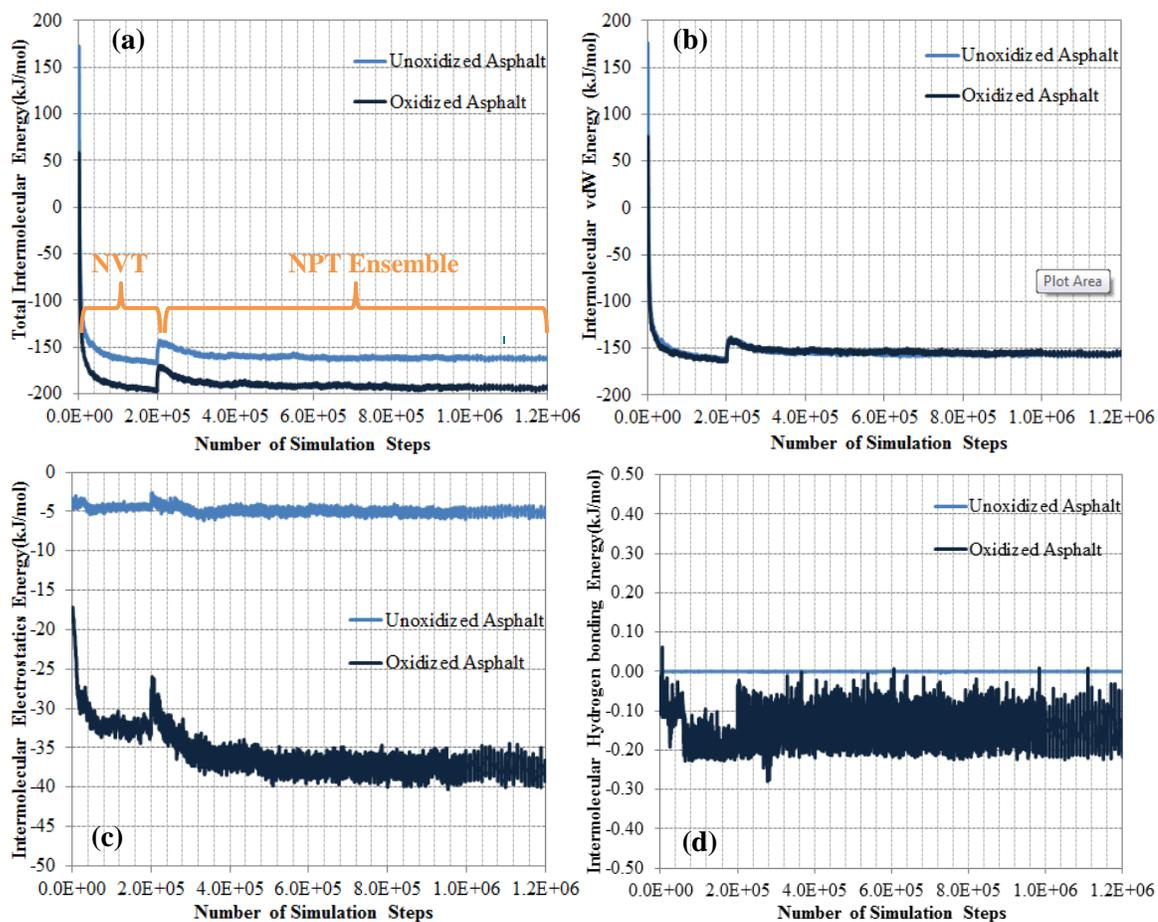
**Figure 4.1** Intermolecular energy changes of asphalt before and after oxidative aging with (a) total intermolecular energy comparison, (b) intermolecular van der Waals energy comparison, (c) intermolecular electrostatics energy comparison, and (d) intermolecular hydrogen bonding energy comparison
