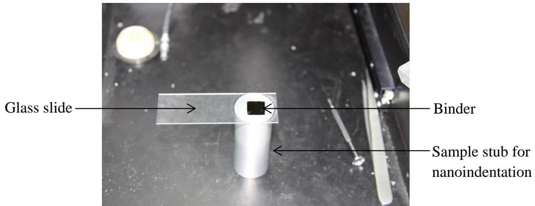
**Figure 7.12** Binder sample prepared for nanoindentation
