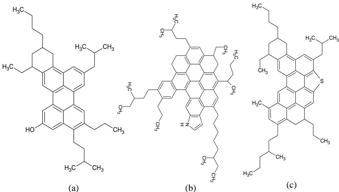
**Figure 2.12** Structures of asphaltenes: (a) asphaltene-phenol, (b) asphaltene-pyrrole, and (c) asphaltene-thiophene (Li and Greenfield 2014)
