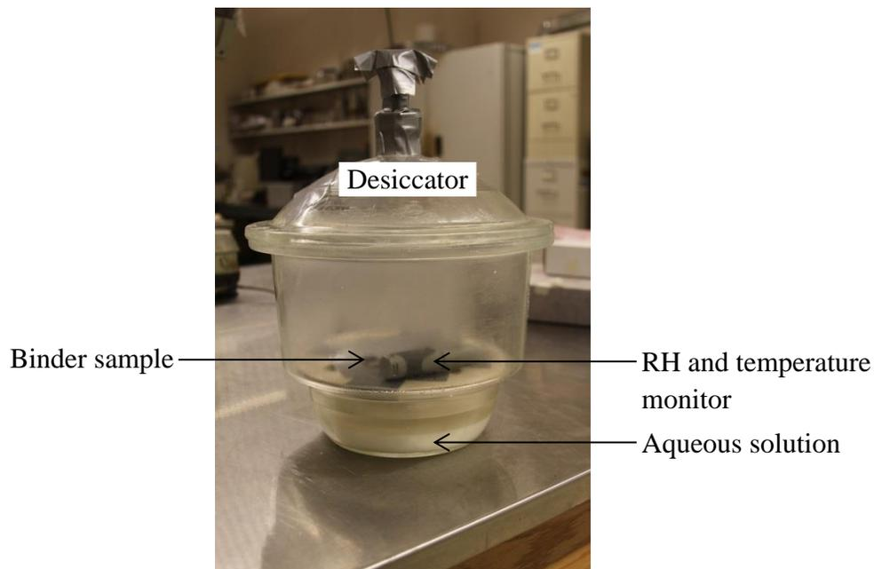
**Figure 7.6** Laboratory setup for moisture conditioning
