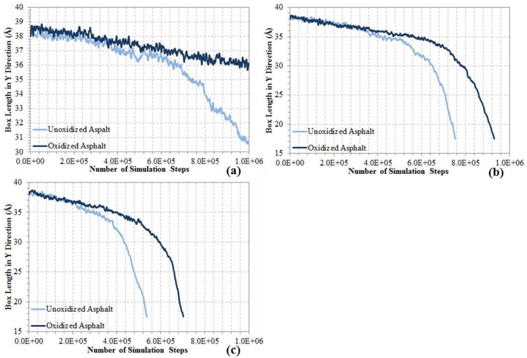
**Figure 5.4** Comparison of unoxidized and oxidized asphalts under different compressive stress rates: (a) 284 GPa sec<sup>-1</sup>, (b) 709 GPa sec<sup>-1</sup>, and (c) 993 GPa sec<sup>-1</sup>
