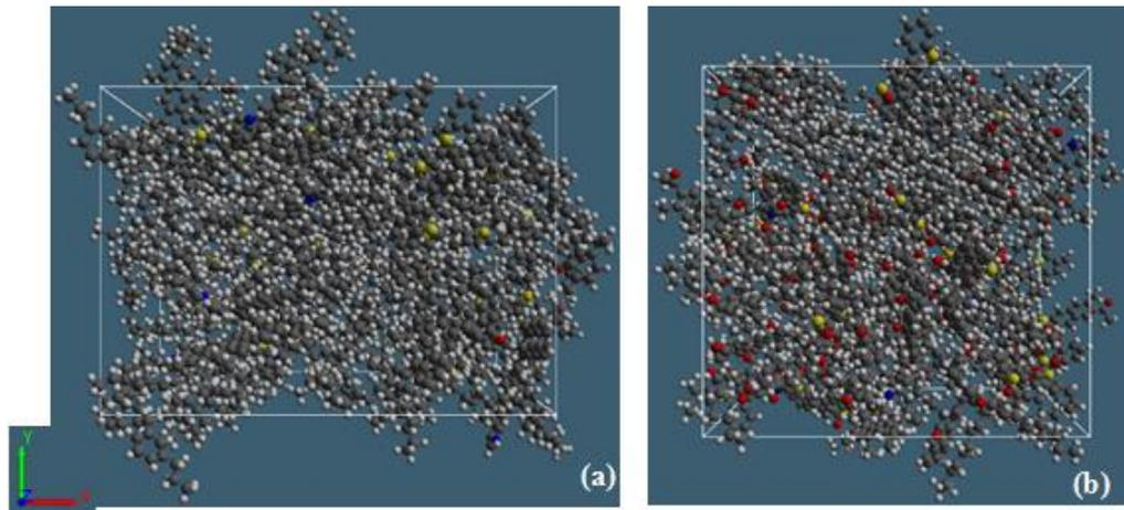
**Figure 5.2** Configurations of asphalt systems before (a) and after (b) oxidation under compressive stress rate of 284 GPa sec<sup>-1</sup>
