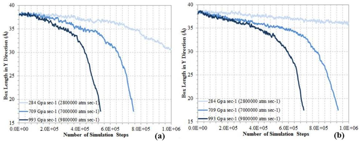
**Figure 5.1** Simulation results of unoxidized and oxidized asphalts under different compressive stress rates in Y direction with (a) unoxidized asphalt and (b) oxidized asphalt
