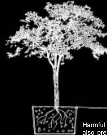
Structural Soil and the trench improve the life and health of the urban street tree by creating necessary voids for air and water pockets for the roots.
