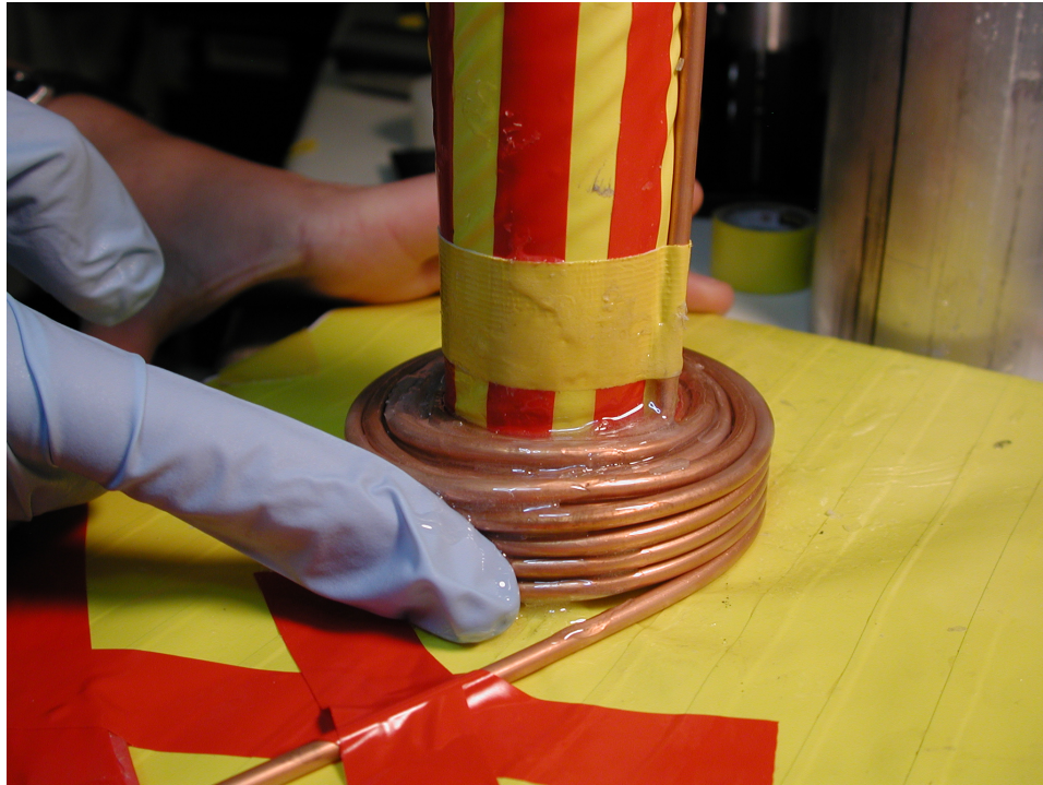
Figure 3.1: Production of an LP magnetic coil. The support and former piece were covered in vinyl electrical tape, since it was found that this was one of the few items available in the lab that the epoxy glue would not adhere to. The adhesive on the back of the tape was scraped off with the help of commercial water-displacing lubricant spray, which was good at un-bonding it from the vinyl. These protective, non-adhesive sheets of vinyl could then be peeled off the formed coil after the epoxy had hardened.
